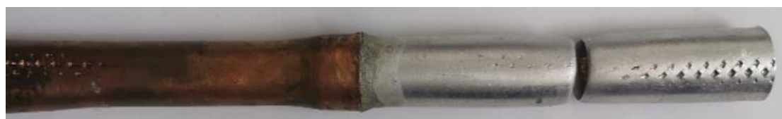
Figure (5): Tensile Testing Specimen Failure at aluminum pipe.
