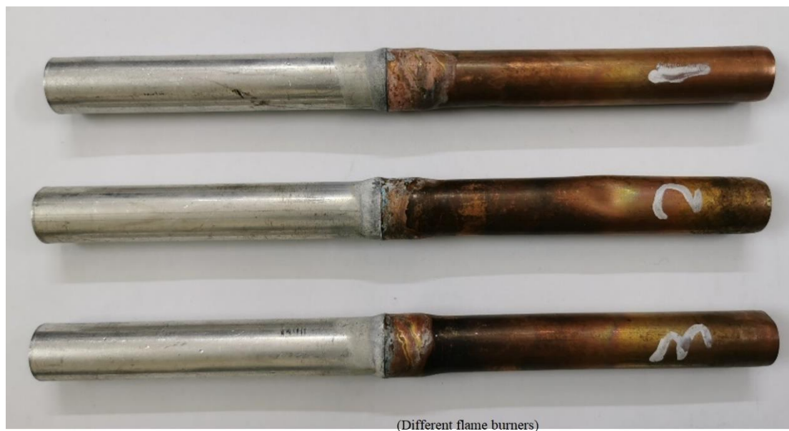
Figure (3): Final Pipe Welding
