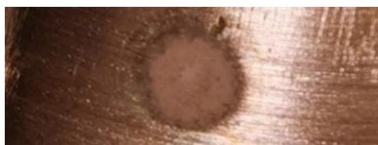
Figure (4): Brinell Hardness Test Indentation
