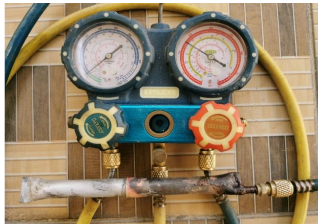
Figure (8). The set up of pressure Test of Welded Specimen
