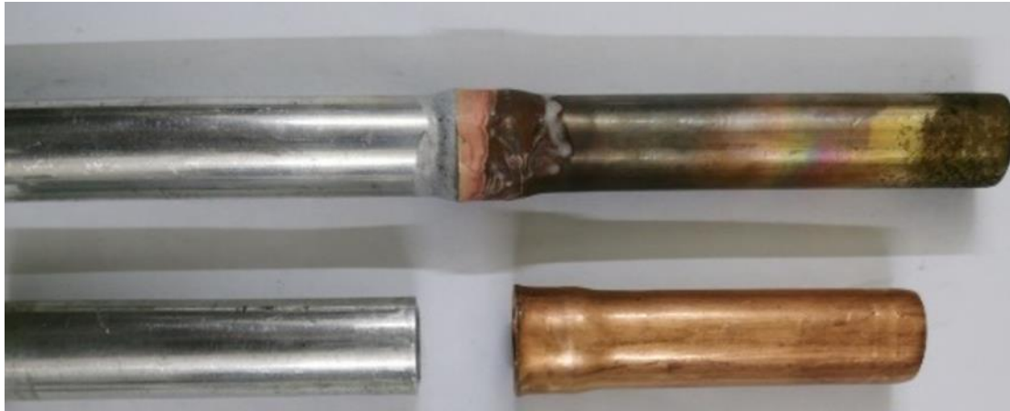
Figure (2): Aluminum to Copper Pipes welding.
