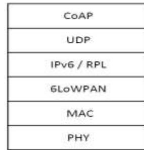
Figure 3: IoT software stack
