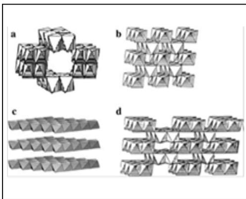
**Figure 1: Sketch diagram of a  $\alpha$ - $\text{MnO}_2$  (Hollandite), b  $\beta$ - $\text{MnO}_2$  (Pyrolusite), c  $\delta$ - $\text{MnO}_2$  (Birnessite), d  $\gamma$ - $\text{MnO}_2$  (Nsutite) [8]**
