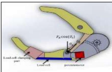
Figure 3: Load cell mounting with hand mechanism
