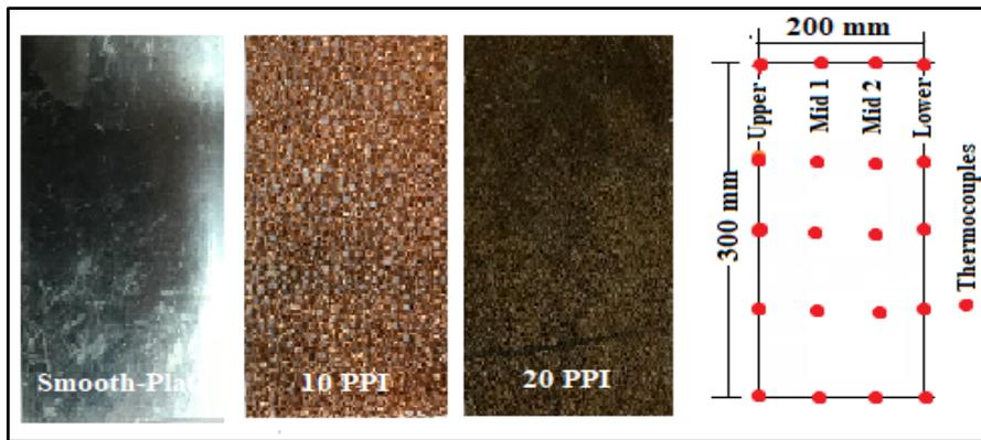
Figure2. Test Plate with CF (10 and 20 PPI) and without CF ( Smooth Plate)
