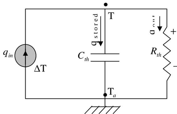
Figure (2) Equivalent electrical circuit of thermal system
