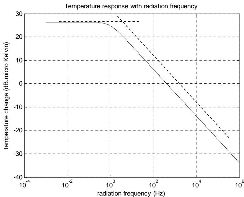
**Figure 8: The temperature response when increasing the radiation frequency in terms of decibel scale from which we see that the corner frequency stays fixed at 1Hz. See the start point of the signal and compare with Fig. 2.**
