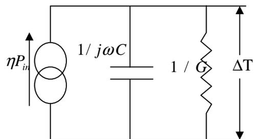
Figure (4) Equivalent electrical circuit of thermal detector model of Fig.3.
