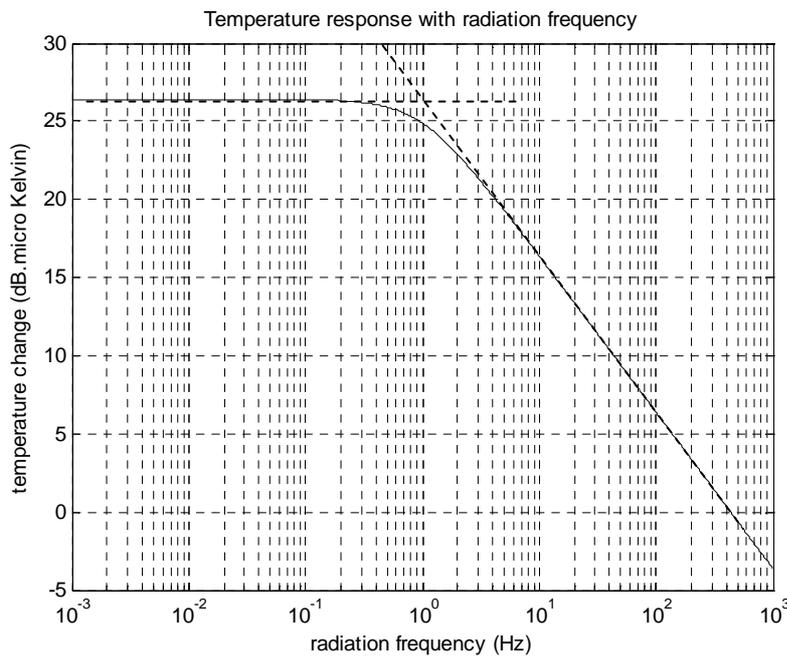
**Figure 6: The decibel concept introduced here to determine the corner frequency at 1 Hz (intersection point of dashed lines) at which the response of thermal detector is start. We see that the temperature change in (dB. Micro Kelvin) versus frequency for the same parameters used simulating Fig.1.**
