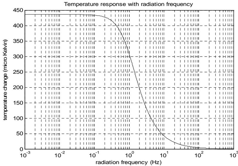
**Figure 5: Temperature change in micro Kelvin against frequency for the interval from  $10^{-3}$  Hz to  $10^3$  Hz of Thermal radiation detector model.**
