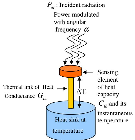
Figure (3) Simplified model of a thermal
