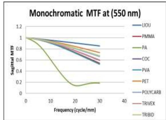
Figure 5: Monochromatic (550 nm) MTF for different materials
