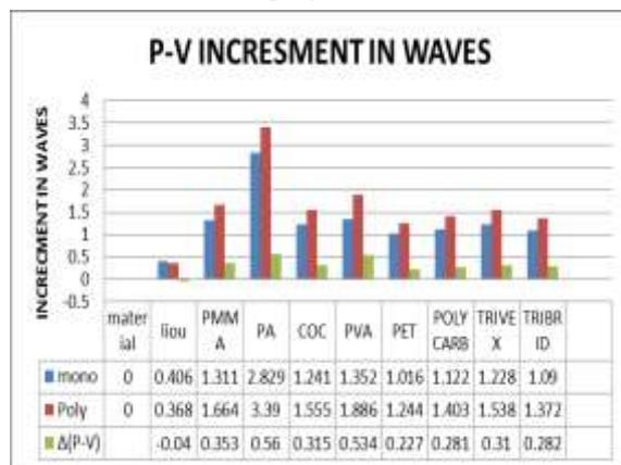
Figure 4: Peak to Valley in waves for Monochromatic light 555nm (Blue), polychromatic light (470-650 nm) (red) and the increment in P-V due to chromatic aberration (green) for different polymer
