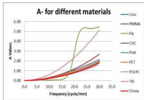
Figure 7: The A-value between polychromatic (470-650 nm) and monochromatic (550nm), Sagittal MTF for the different materials.
