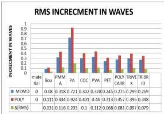
Figure 3: RMS wavefront error for Monochromatic light 555nm (Blue), polychromatic light (470-650 nm) (red) and the increment in RMS due to chromatic aberration (green) for different polymer
