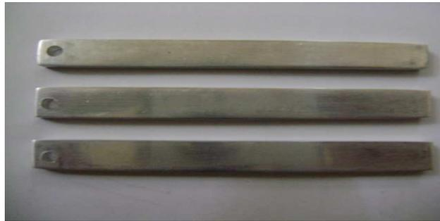
Figure (1): Fatigue test Specimens.
