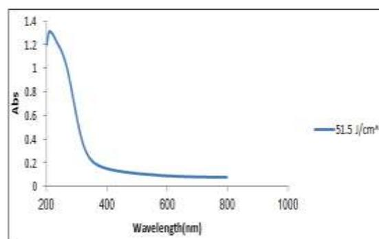
**Figure 4: The absorption spectrum of TiO<sub>2</sub> NPs at 200 pulse, repetition rate=1 Hz, λ=1064nm and 43.4 JL/m<sup>2</sup> fluence**
