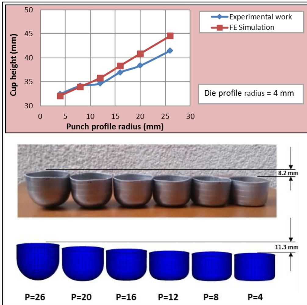
Figure 12: Effect of Punch and Die Profile Radii on the Height of Produced Cup (Comparison of Experimental Work and FE Simulation).
