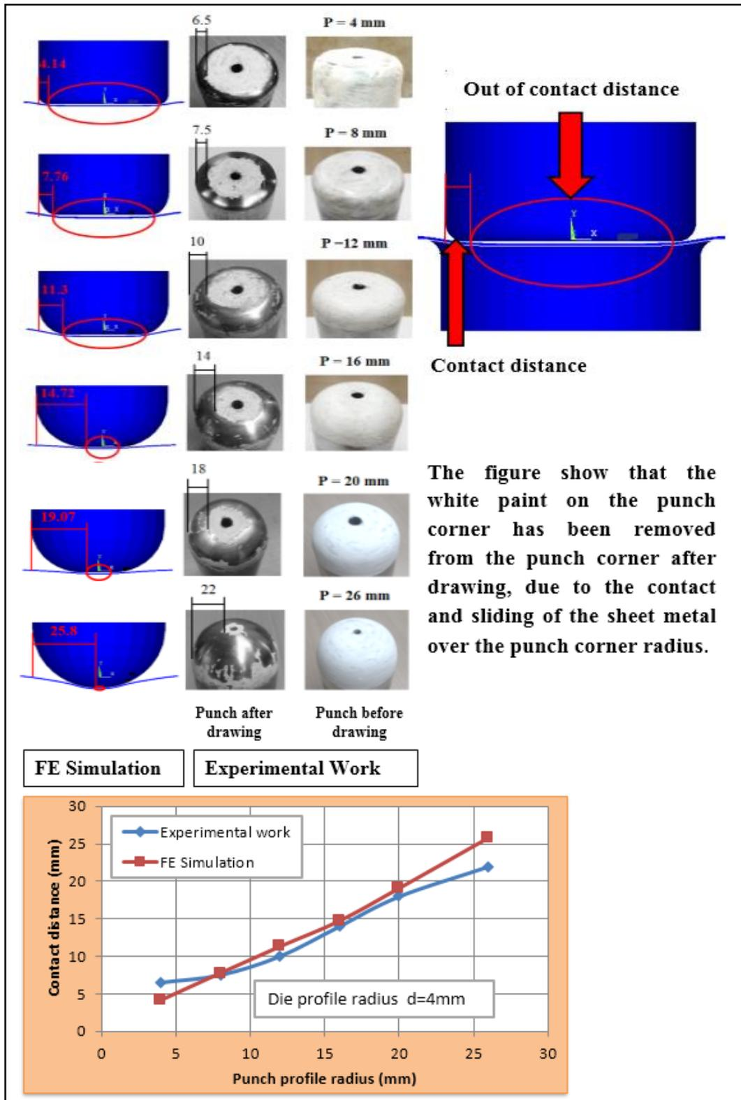
Figure 7: Effect of Punch Profile Radius on Length of Contact Distance between Punch and Blank (Comparison of Experimental Work and FEM).
