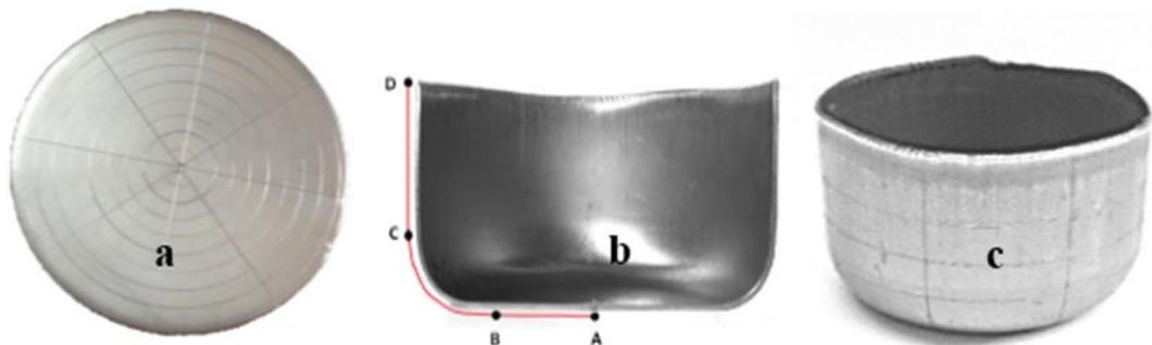
Figure 4: a- Blank with a Circular Grid Pattern, b- Half of a Drawn Cup, c- Completely Drawn Cup.
