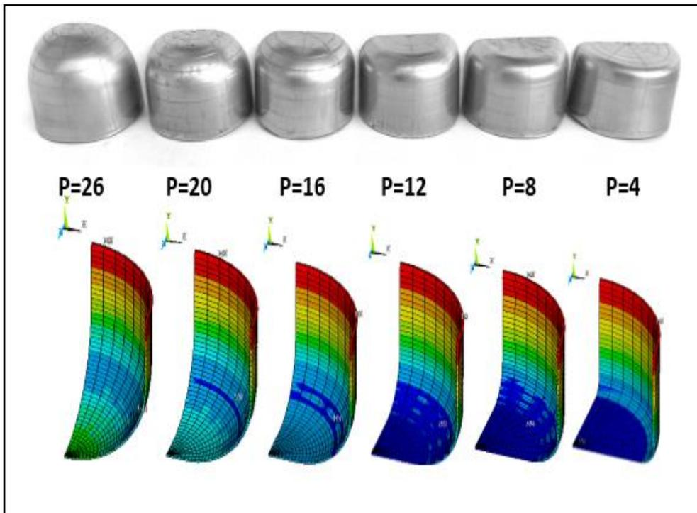
Figure 6: Produced Cups with Various Punches Profiles Radii by both Experimental Work and FE Simulation.
