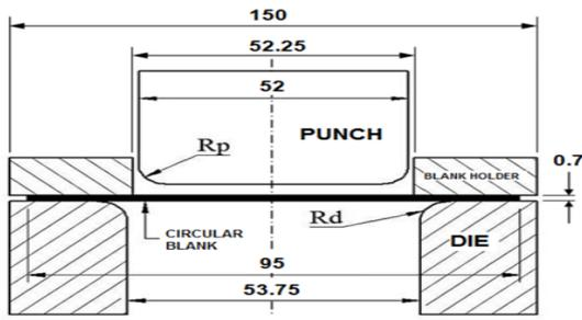
Figure 1: Geometry of the Drawing Tools (Dimensions in mm).
