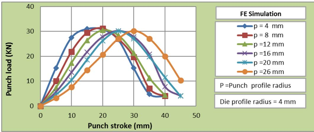
Figure 5: Effect of Punch Profile Radius on Punch Load (Comparison of Experimental Work and FE Simulation).
