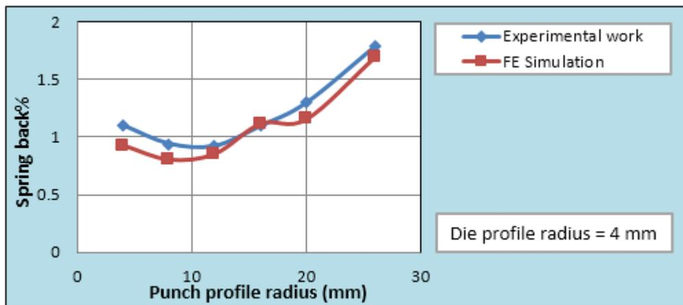
Figure 13: Effect of Punch Profile Radius on the Amount of Spring Back Induced in the drawn Cup (Comparison of Experimental Work and FE Simulation).
