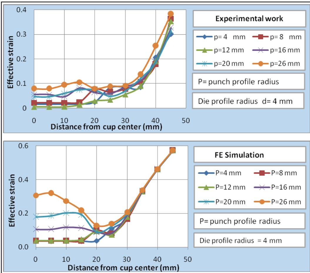
Figure 10: Effect of Punch Profile Radius on Effective Strain (Comparison of Experimental Work and FE Simulation).
