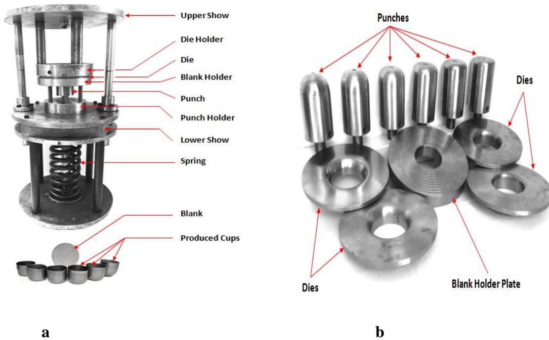
Figure 3: a-Drawing Die Assembly, b-Tools Used in the Experimental Work.
