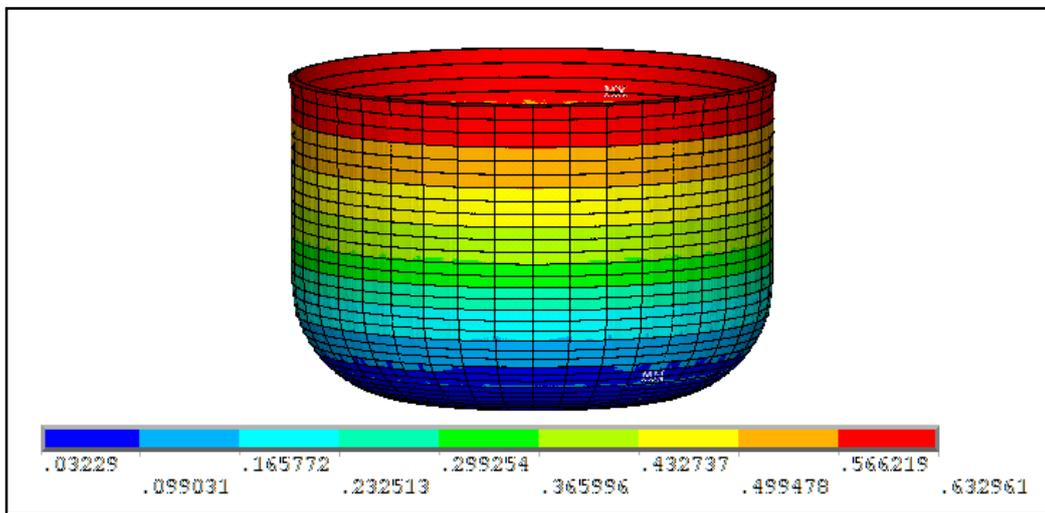
Figure 11: Effective Strain Distribution on the Completely Drawn Cup Produced by FE Simulation with Tools of ( $R_p=12$  mm &  $R_d=4$  mm).
