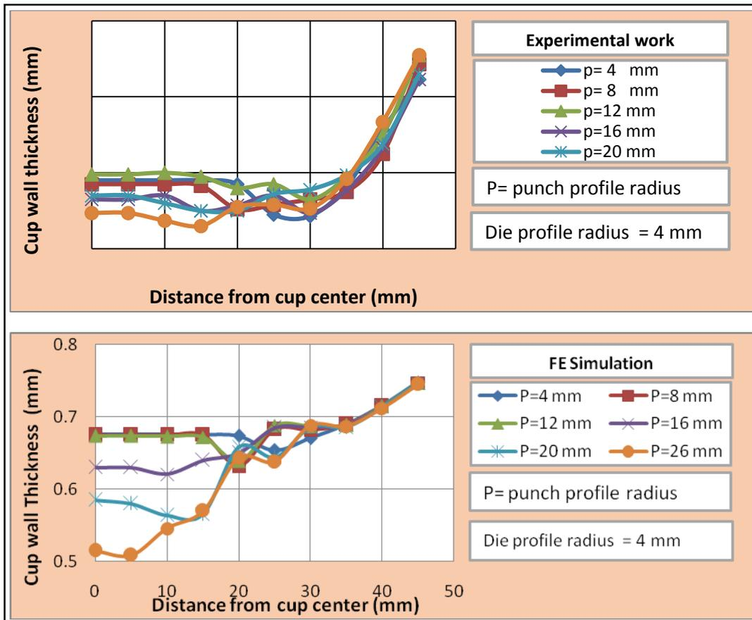
Figure 8: Effect of Punch Profile Radius on Cup Wall Thickness (Comparison of Experimental Work and FE Simulation).
