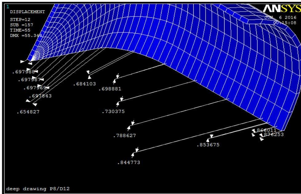
Figure 9: Thickness Variation over the Produced Cup Wall Obtained by FE simulation.
