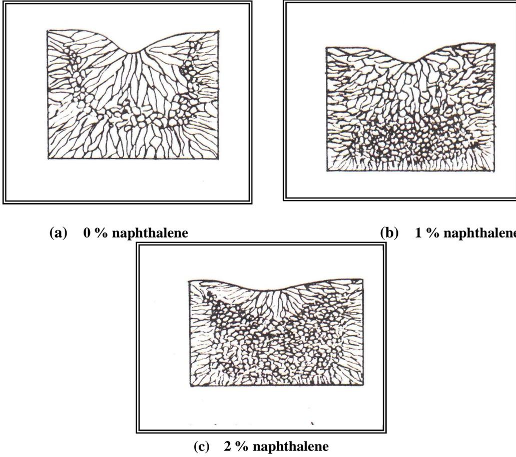
Figure (1) Ingot structure of commercially pure aluminum with different naphthalene additions.
