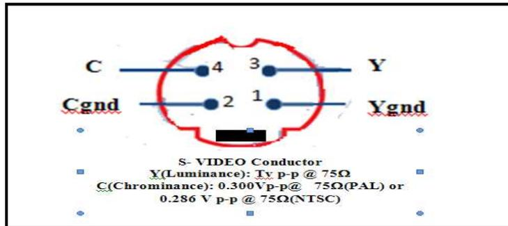
Figure (1) The Pin Connections for the 4 – Pin mini DIN connector used for most S – video cables [5]
