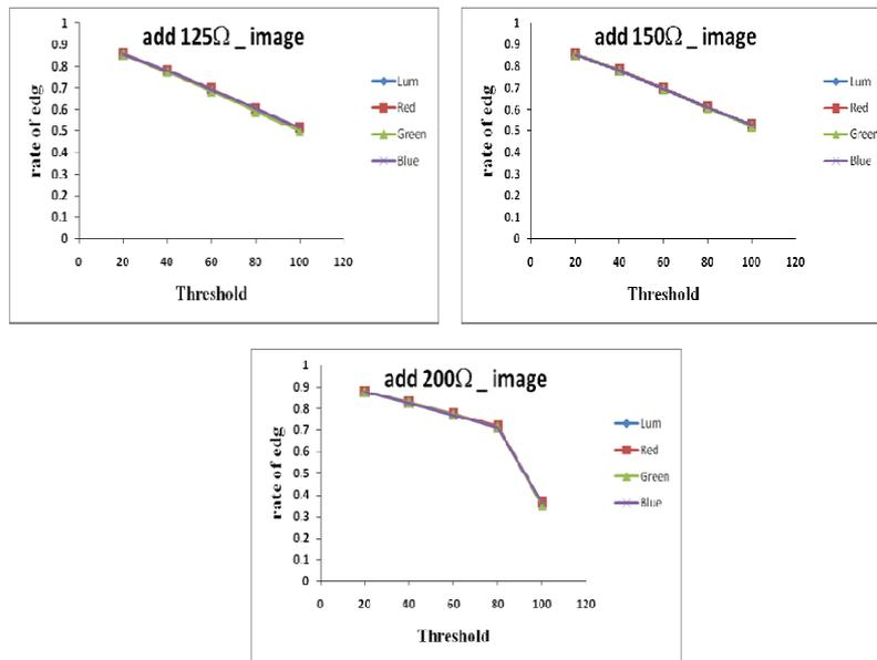
Continuo Figure(8) shows the rate of edge point of the original image and different image which used resistance(75,125,150, 200) $\Omega$  in the cable signal transfer video for (L- RGB) components of each image for different threshold
