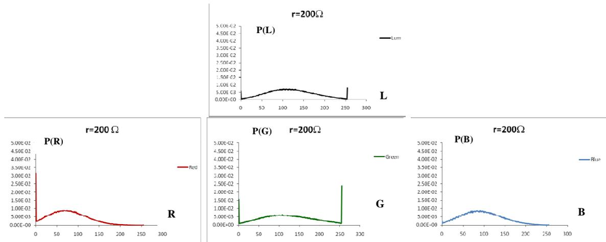
Continue Figure( 5) shows the histogram of the image which used resistance( $200\Omega$ ) in the cable signal transfer video for (L-RGB) components of each image
