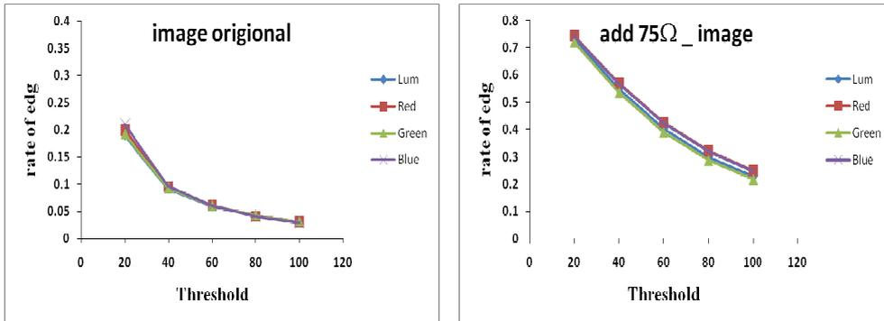
Figure (8) shows the rate of edge point of the original image and different image which used resistance(75,125,150, 200) $\Omega$  in the cable signal transfer video for (L- RGB) components of each image for different threshold
