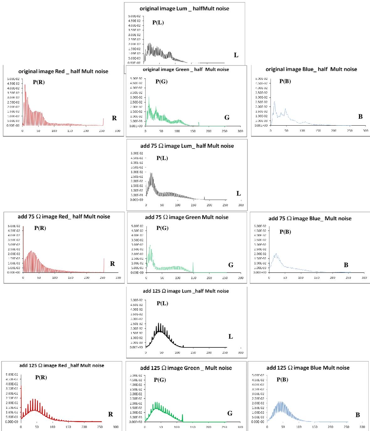
Figure(7) shows the histogram to half multiplicative noise of the image original and image which used resistance(75,125) $\Omega$  in the cable signal transfer video for (L-RGB) components of each image
