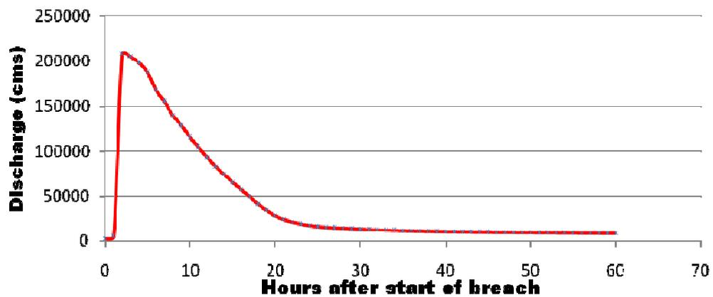
Figure (4) upstream discharge hydrograph (after Swiss consultant 1985)
