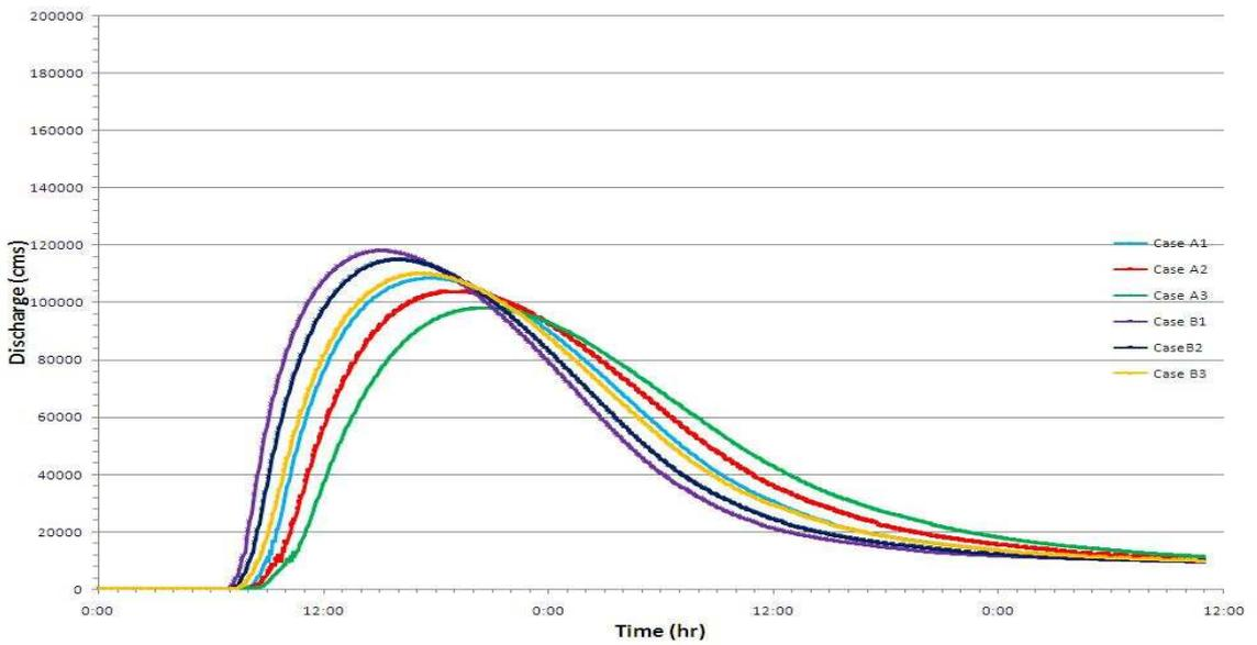
Figure (8) The peak flow and travel time of flood wave at Hit city
