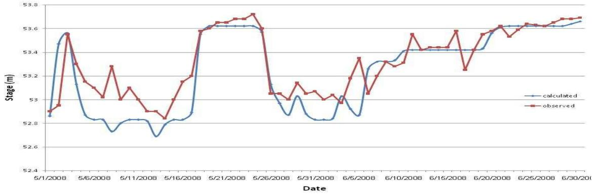
Figure (7) Observed and calculated stage of the Euphrates River at Hit gage station
