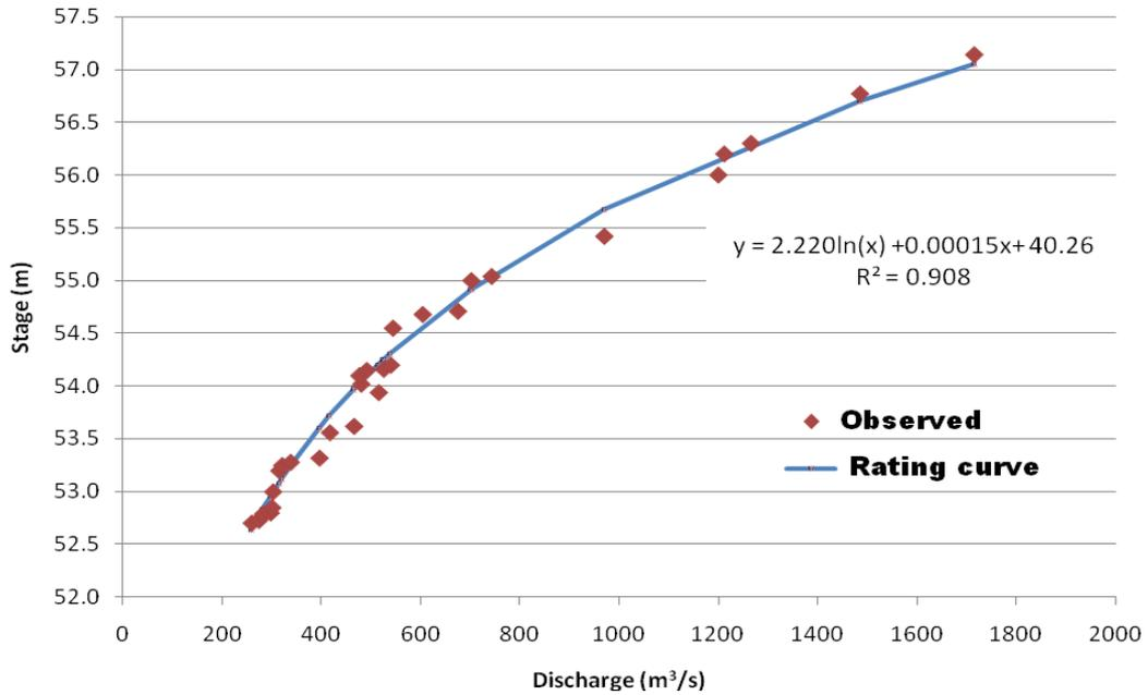
Figure (5) Rating curve at Hit gauge station, after head office of Al-Ramadi barrage (2008)
