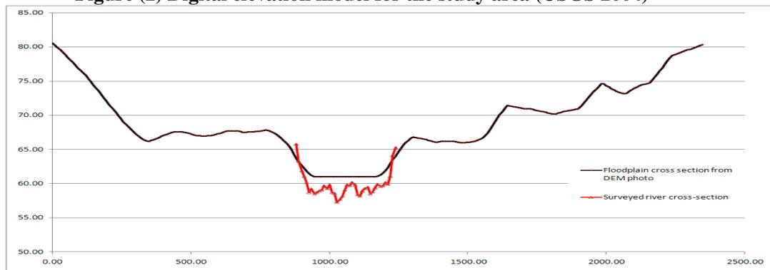
Figure (3) Surveyed cross-section of Euphrates River superimposed to (DEM) data
