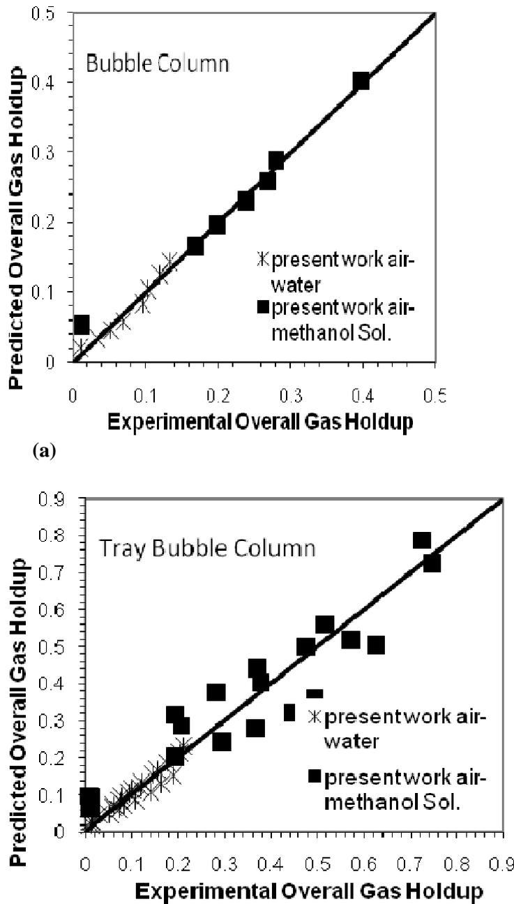
(b) Figure (5) Comparison between the experimental and prediction correlation data of this work in (a) bubble column (b) tray bubble column
