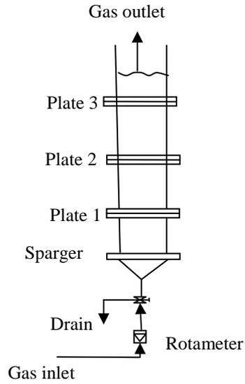
**Figure (1) Tray bubble column experimental setup**
