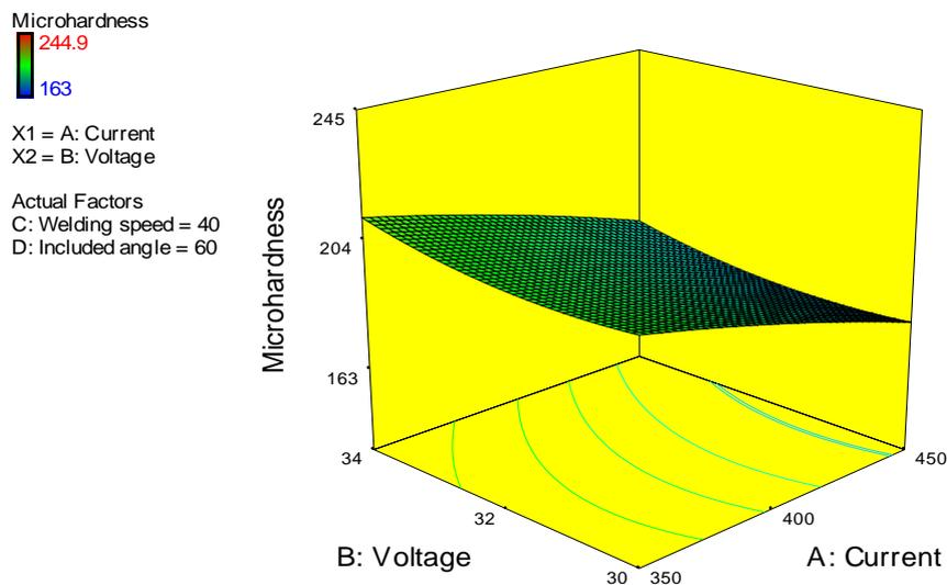
Figure 9: Three-dimensional plot of microhardness in terms of voltage and current at the center level ((60°) included angle and (40 cpm) welding speed).
