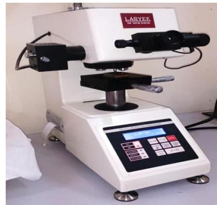
Figure 3: Digital microhardness tester
