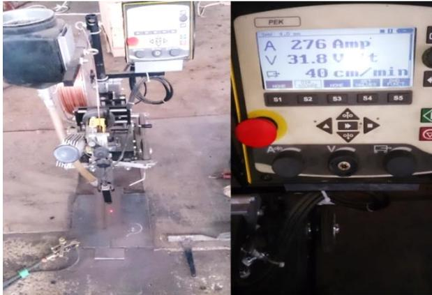
Figure 2: A view of Esab A2 Multitrack welding machine with the A2-A6 process controller PEK
