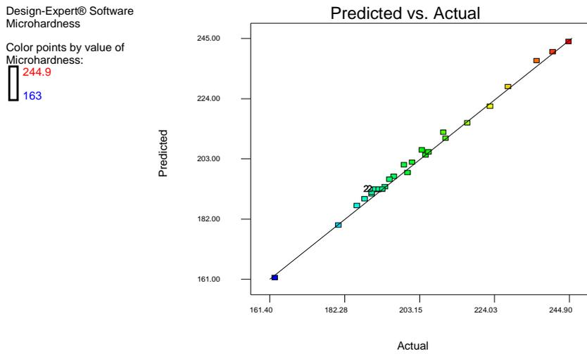
Figure 6: Predicted vs. actual microhardness results for comparison.
