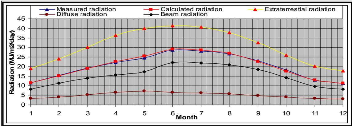
Figure (1a) Monthly average daily, Measured global radiation, calculated global radiation, extraterrestrial radiation diffuse radiation, and beam radiation for Baghdad city.
