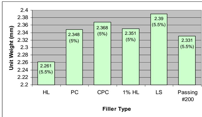
Figure (7) Maximum Unit Weight Versus Filler Type (number between parenthesis refers to binder content that provides the maximum unit weight).
