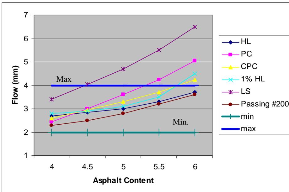
Figure (3) Marshall Flow versus Asphalt Content.
