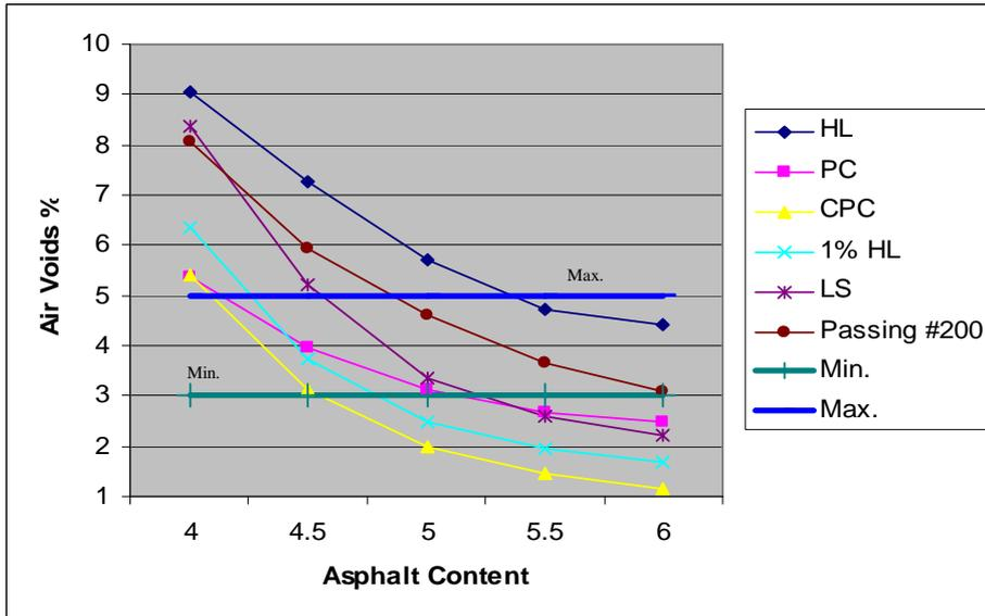
Figure (4) Voids in Total Mix versus Asphalt Content.
