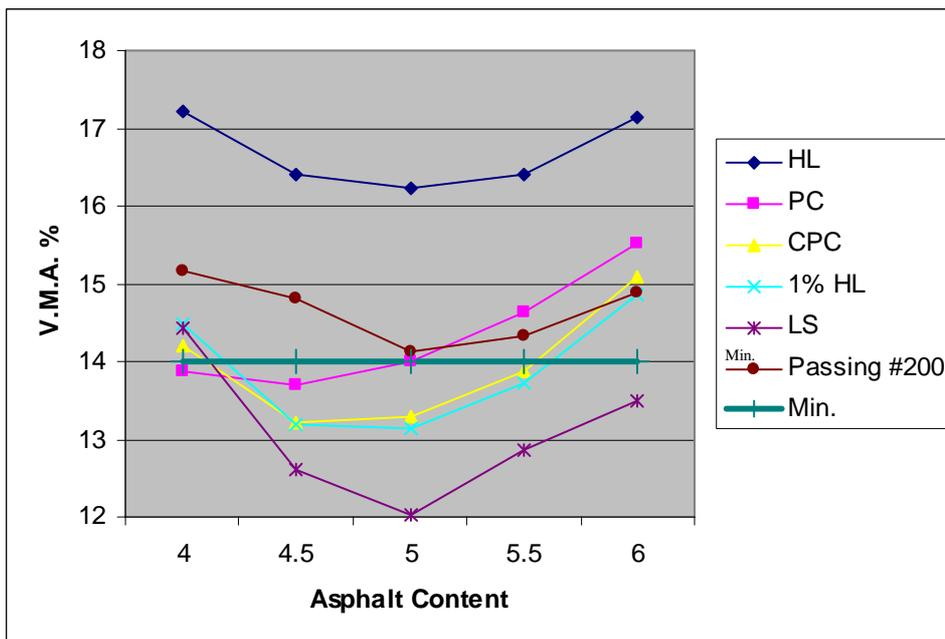
Figure (5) Voids in Mineral Aggregate versus Asphalt Content.
