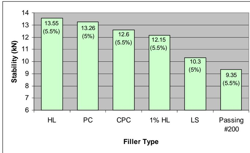
Figure (8) Maximum Stability Versus Filler Type (number between parenthesis refers to binder content that provides maximum stability)
