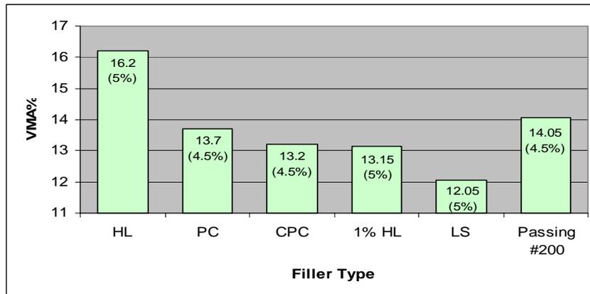
Figure (11) Minimum VMA Versus Filler Type (number between parenthesis refers to binder content that provides minimum VMA).
