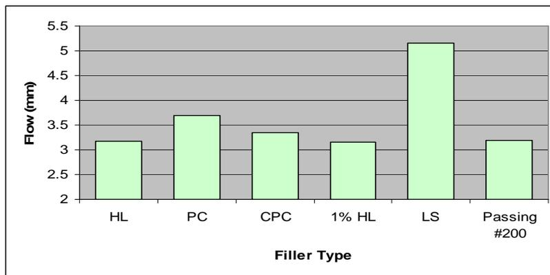
Figure (9) Median Flow Versus Filler Type.
