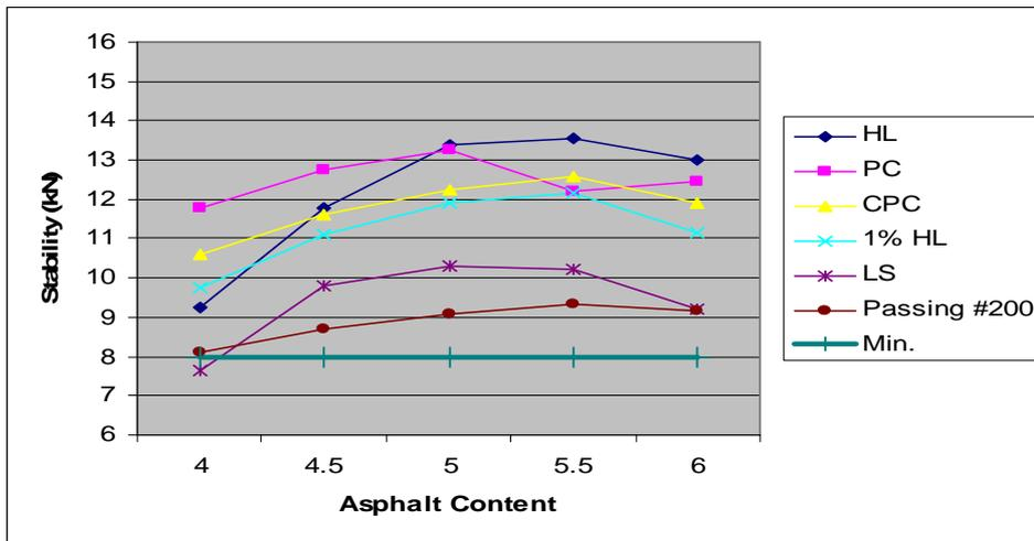
Figure (2) Marshall Stability versus Asphalt Content.
