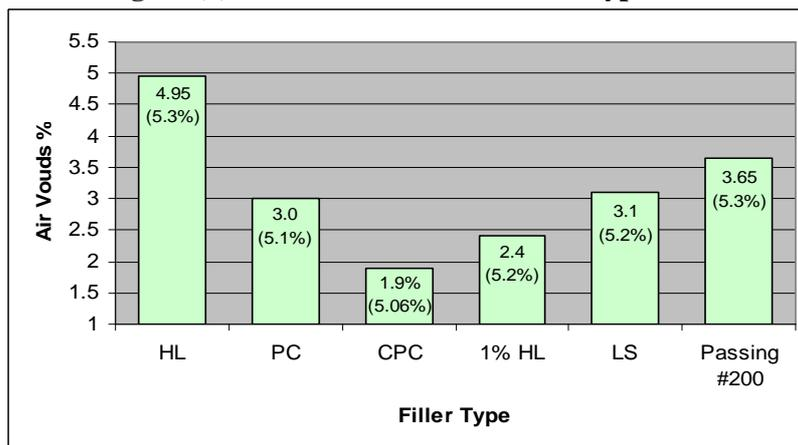
Figure (10) Median Voids in Total Mix Versus Filler Type (number between parenthesis refers to binder content that provides median voids in total mix ).
