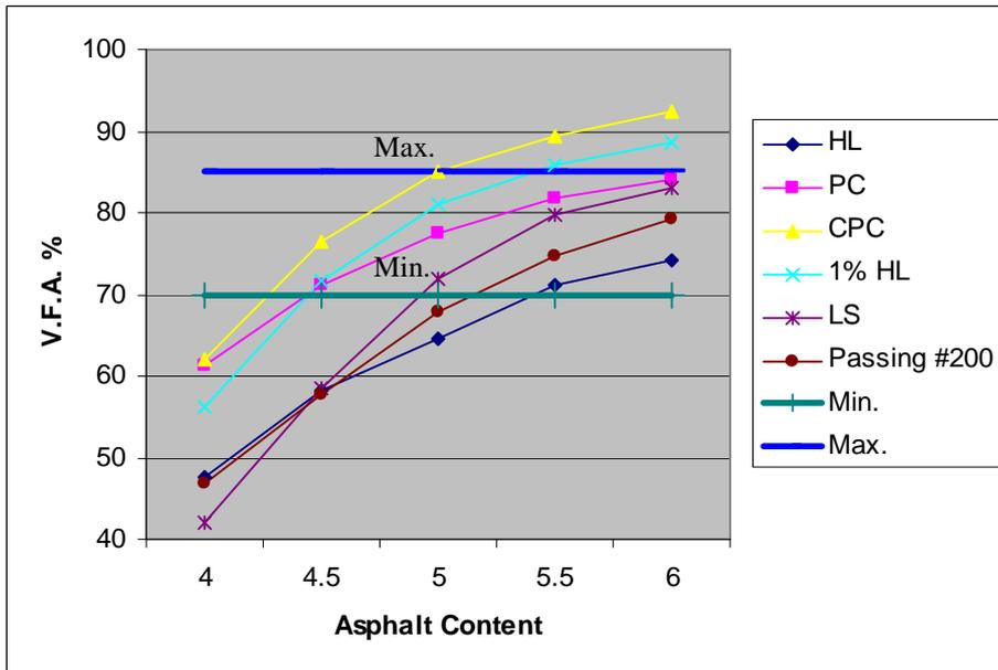
Figure (6) Voids Filled with Asphalt Versus Asphalt Content.
