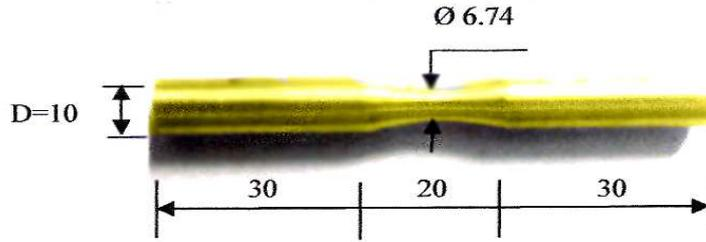
Figure (1) : shows the geometry of fatigue creep interaction specimens, dimensions in (mm)
