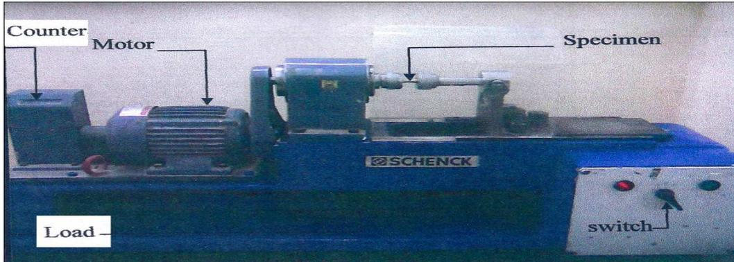
Figure (2): PUNN Rotary Fatigue bending machine [8]
