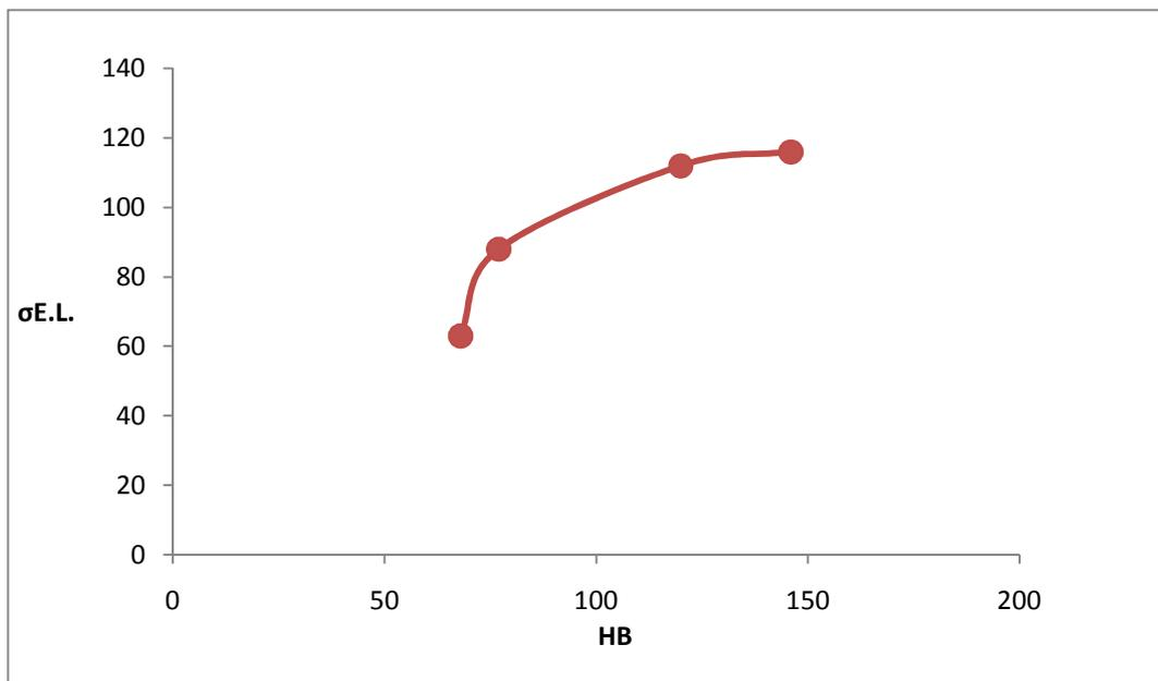
Figure (5) Fatigue strength against HB at different temperatures (room temperature to 300°C)
