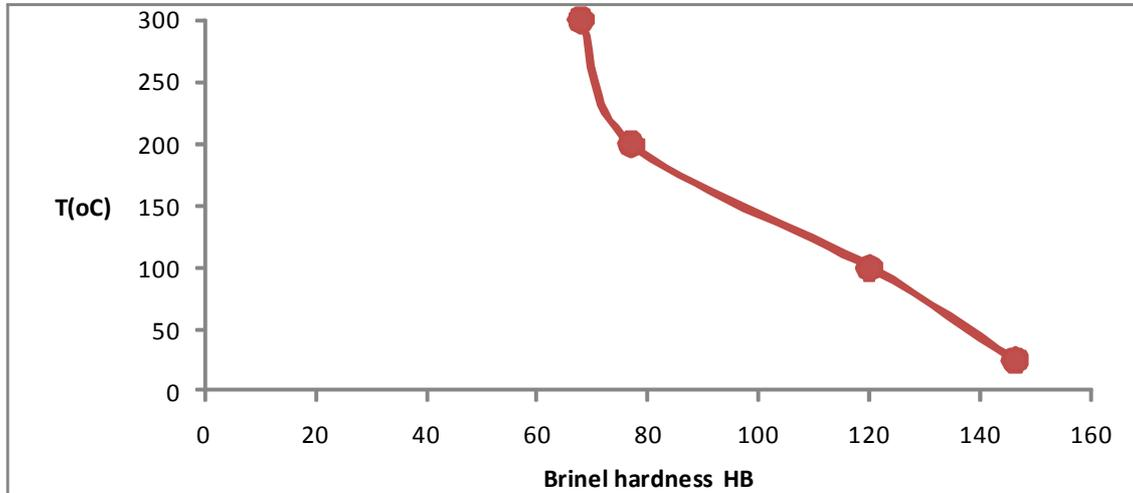
Figure (4-B) shows the variation of temperature with the HB hardness of copper alloy
