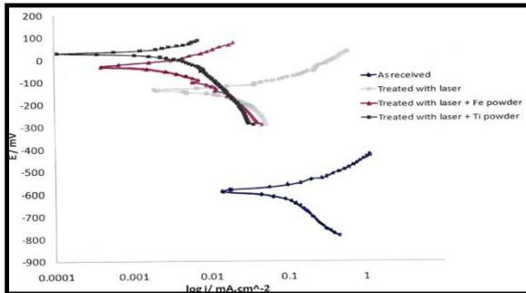
Figure 5: Potentiodynamic polarization for] base and laser treatments 1000 kJ.
