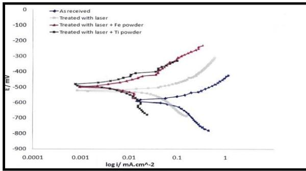
Figure.4: Potentiodynamic polarization for as received and laser treatments 750 kJ.
