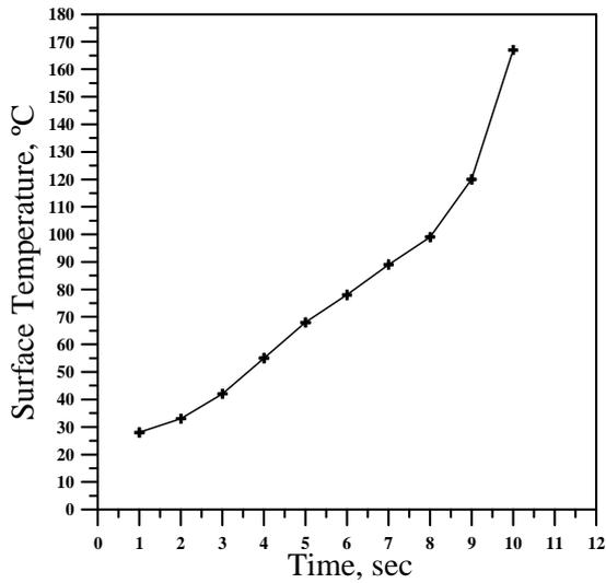
figure (5): Variation of surface temperature Vs time of exposed to flame at exposed distance (10 mm)
