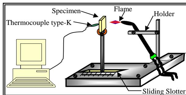
Figure (3): Mechanism of thermal erosion
