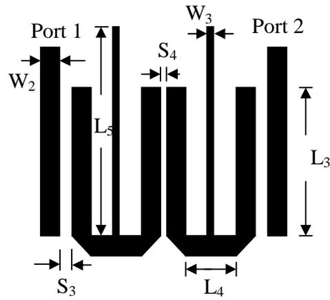
Figure (2) Topology of the proposed bandpass filter
