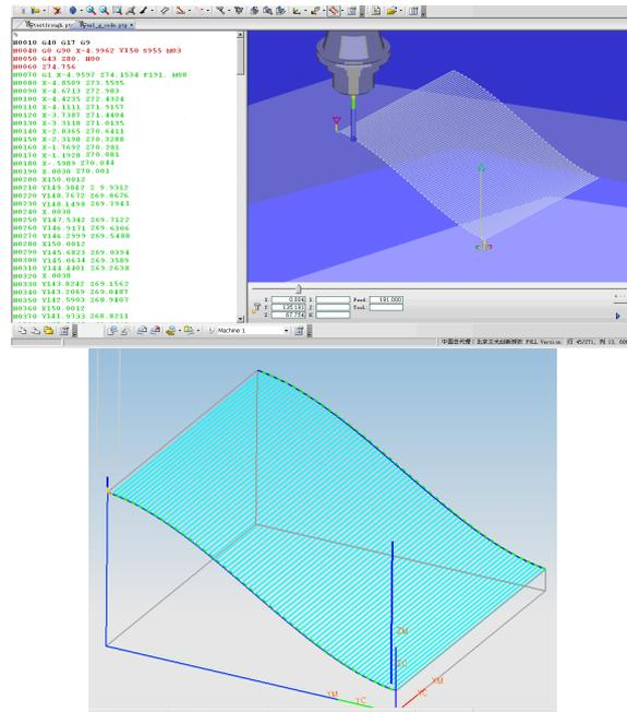
Figure (6) UG-NX5 Main window while managing 1<sup>st</sup> parametric surface
