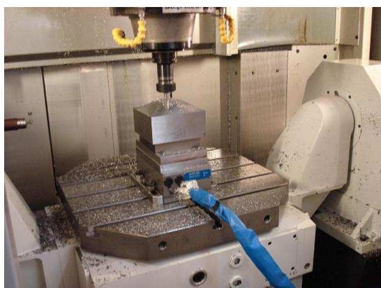
**Figure (8) The finished Machined Parametric Surface No.2**
