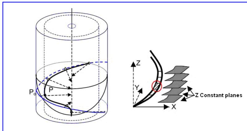
Figure (1) Cutting edge discretization [12]
