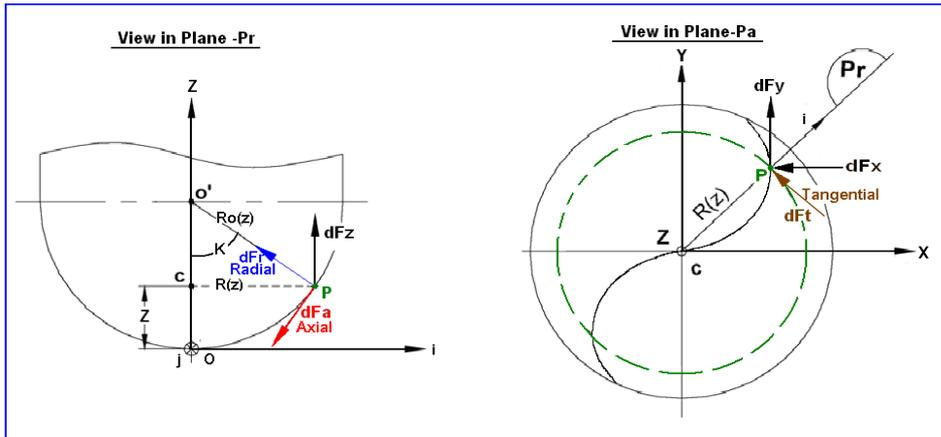
Figure (2) Elemental Cutting Forces
