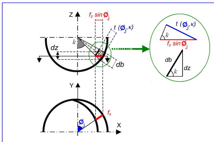
Figure (4) Un-cut chip thickness
