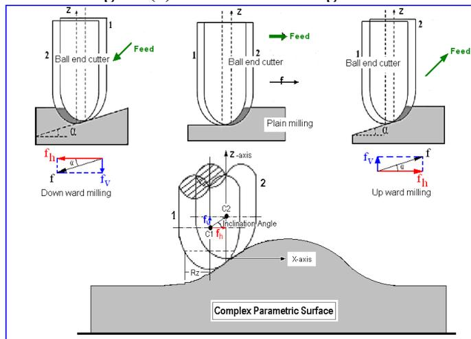
Figure (3) downward Milling, Upward Milling and Plain Milling cases in Machining Parametric surface
