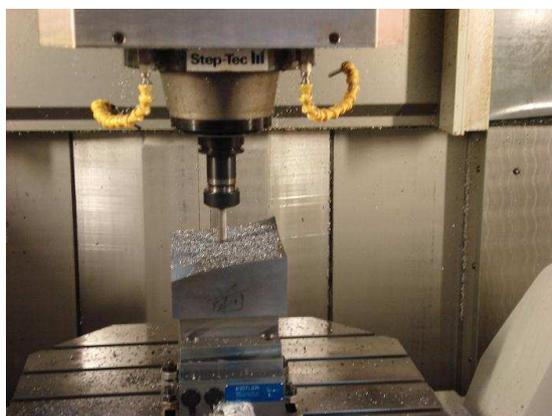
**Figure (9) The finished Machined Parametric Surface No.3**
