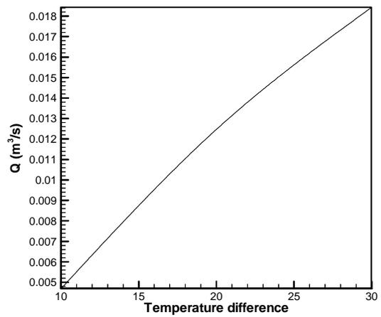
**Figure8:** The relation between induced flow rate with the temperature difference of the walls.
