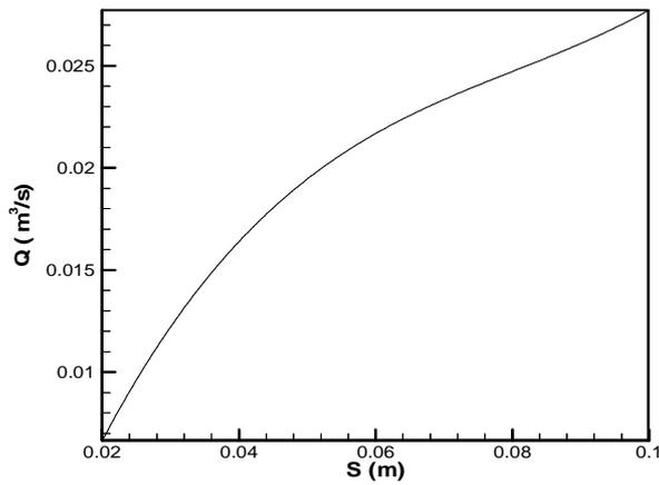
**Figure 9:** The relation between induced flow rate with the width of the channel.
