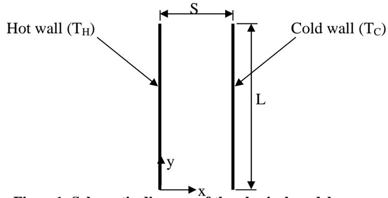
Figure1: Schematic diagram of the physical model.
