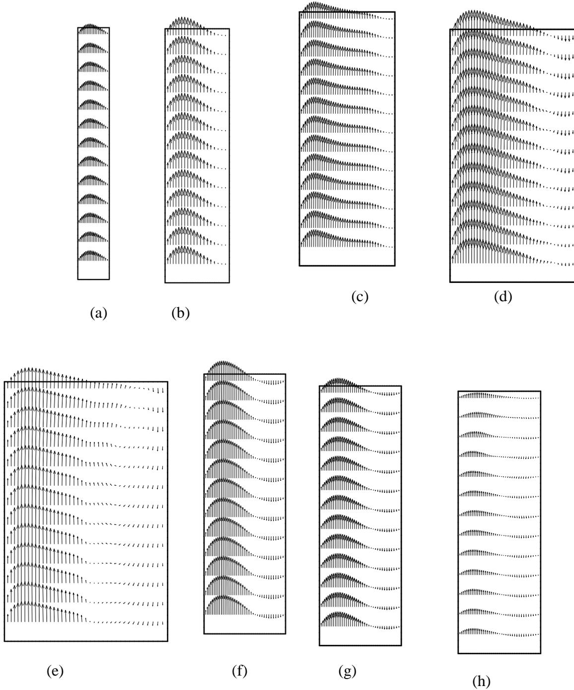
Figure 5. Velocity vector within the channel at  $\Delta T = 30$  for (a)  $A=20$ , (b)  $A=10$ , (c)  $A=6.6$ , (d)  $A=5$ , (e)  $A=4$ , and  $\Delta T = 30, 20$  and  $10$  for  $A=8$  in f, g and h respectively.
