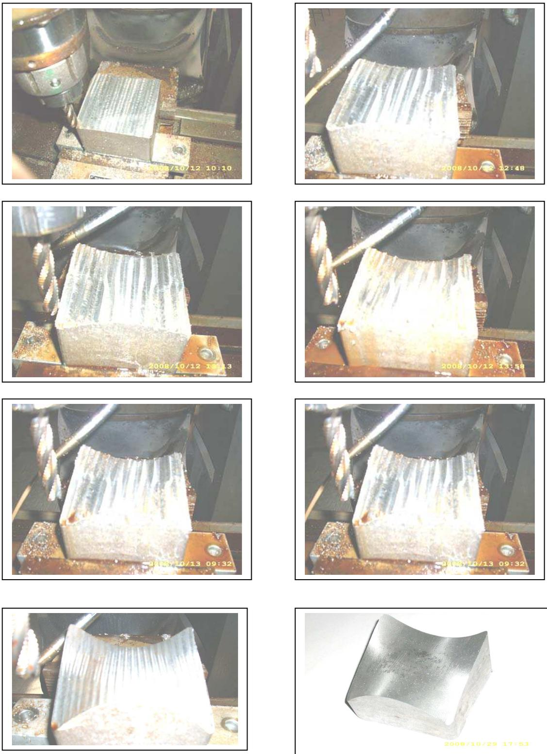
Figure 13. Various machining stages of the 3rd sculptured surface
