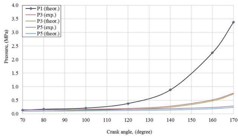
**Figure (21) Theoretical and experimental results of pressures inside the inter-ring crevices region  $P_1$ ,  $P_3$ & $P_5$  as functions of crank angle case (III)**
