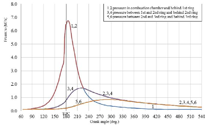
**Figure (12) Pressure distributions between and behind piston rings as functions of crank angle case (I) . N =2200 rpm**
