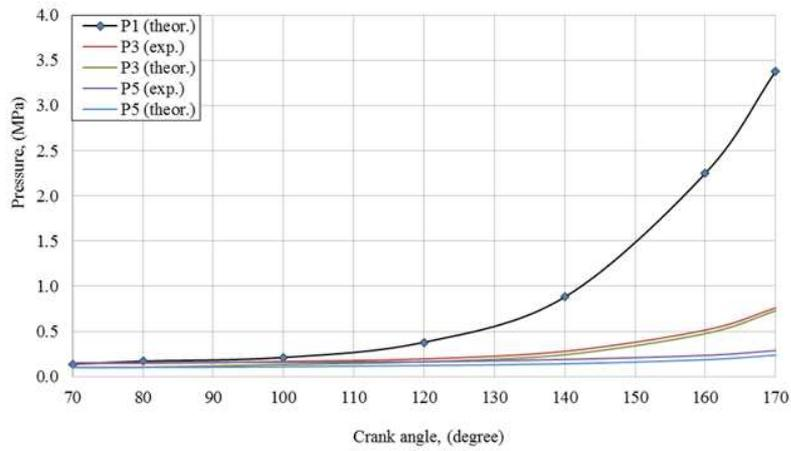
**Figure(20) Theoretical and experimental results of pressures inside the inter-ring crevices region  $P_1$ ,  $P_3$ & $P_5$  as functions of crank angle case (II)**
