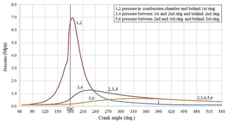
Figure (10) Pressure distributions between and behind piston rings as functions of crank angle case (I) , N =1200 rpm
