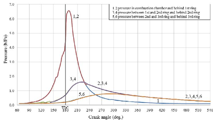
Figure (16) Pressure distributions between and behind piston rings as functions of crank angle case (III), N =1200 rpm
