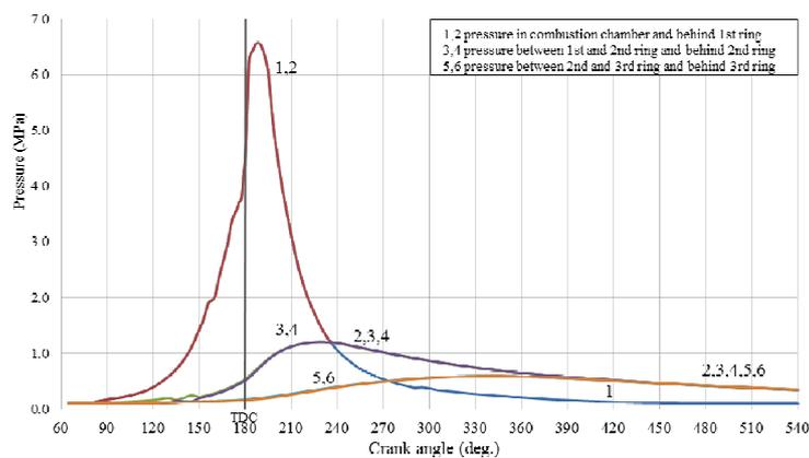
**Figure (13) Pressure distributions between and behind piston rings as functions of crank angle case (II) N =1200 rpm**
