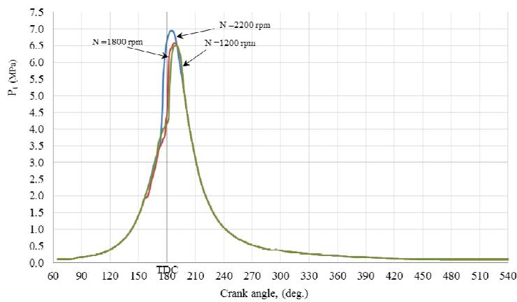
**Figure(7) Pressure indicator diagram of as a function of crank angle , case I**
