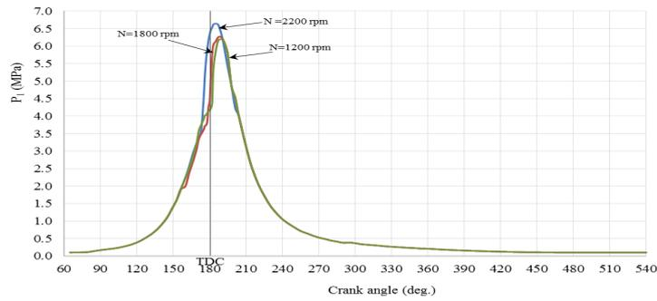
Figure (8) Pressure indicator diagram of as a function of crank angle , case II
