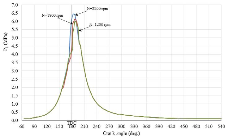
Figure (9) Pressure indicator diagram of as a function
