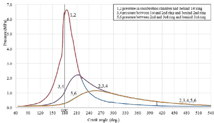
Figure(15) Pressure distributions between and behind piston rings as functions of crank angle case (II), N =2200 rpm
