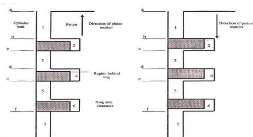
**Fig. (3.1): Schematic Diagram for the Gas Flow Through Piston Rings [9].**
