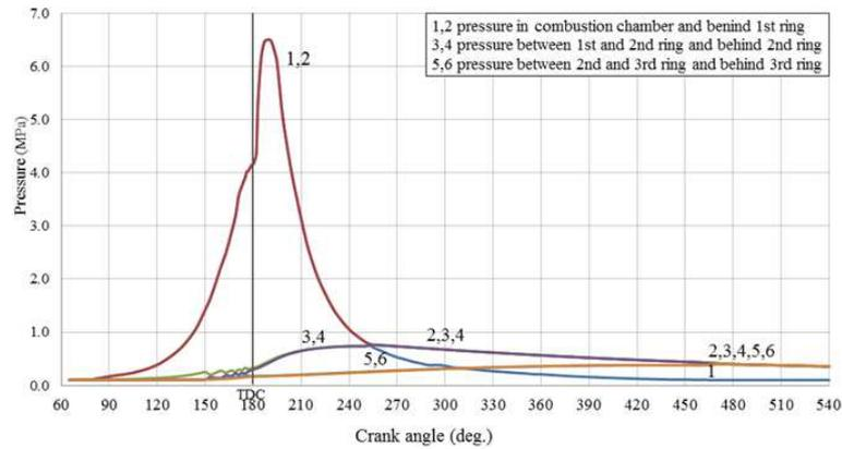
**Figure (11) Pressure distributions between and behind piston rings as functions of crank angle case (I) , N =1800 rpm**
