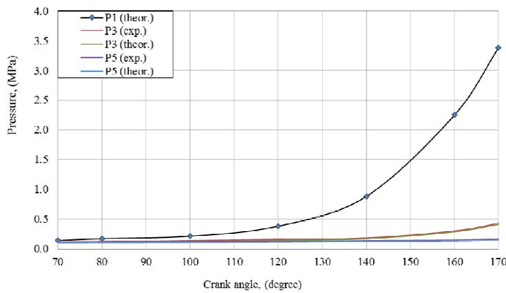
Figure(18) Pressure distributions between and behind piston rings as functions of crank angle case (III) , N =2200 rpm
