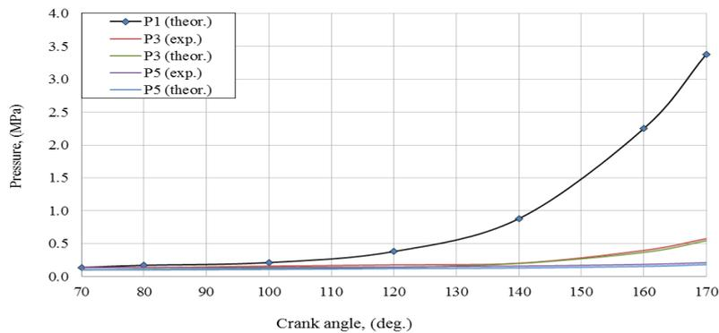
Figure (19) Theoretical and experimental results of pressures inside the inter-ring crevices region P<sub>1</sub>, P<sub>3</sub>&P<sub>5</sub> as functions of crank angle case (I)
