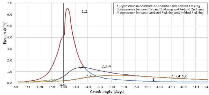
Figure (17) Pressure distributions between and behind piston rings as functions of crank angle case (III) , N =1800 rpm
