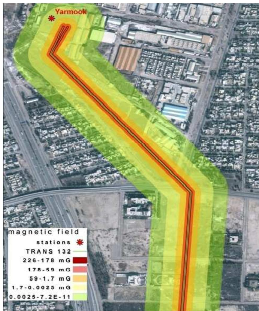
Figure (6) The Magnetic Field Buffers Layer
