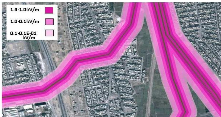
Figure (7) The electric field buffers layer
