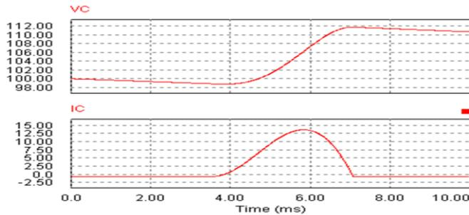
Figure (3): Imaginary voltage and current waveforms for  $C=2\text{mF}$ ,
