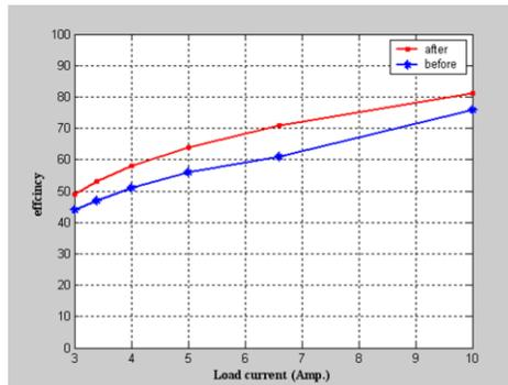
Figure(18): Variations of efficiency power before and after filter due to the variation of secondary currents.
