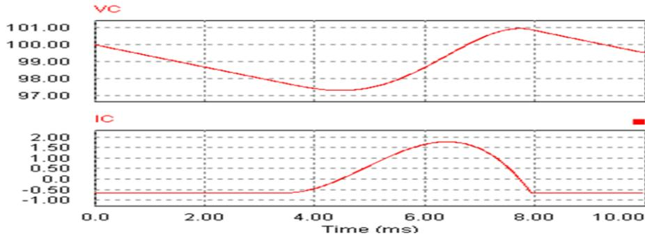
Figure (5): Imaginary voltage and current waveforms for  $C=1\text{ mF}$ ,  $L=5\text{mH}$  and  $R1=150\Omega$
