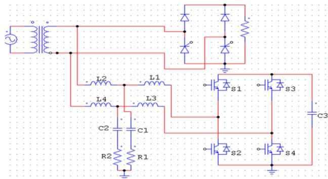
Figure(7): Two branches active filter, transformer, voltage source and rectifier load.
