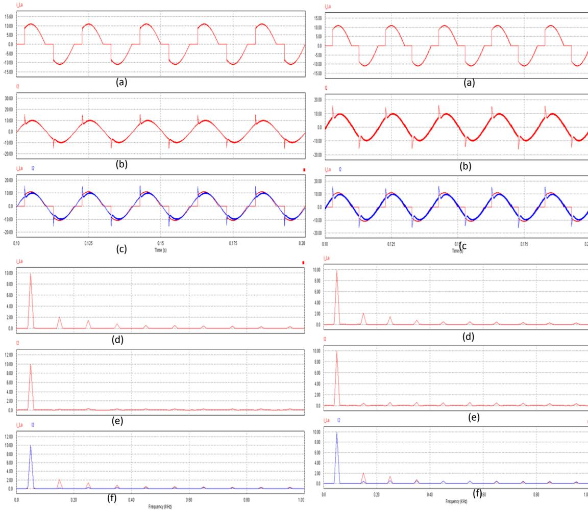
**Figure(14): (a)secondary current before filtered. (b)secondary current after filtered. (c)the compaction between secondary currents by using Fig.6a. Two branches active filter. (d, e and f) Showing the spectrums for the secondary currents before, after filtered and compaction between them, respectively.**
