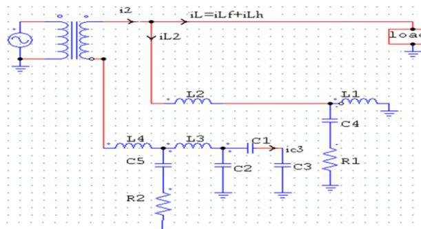
Figure (11): Equivalent circuit of the system and Fig. 6b in the case of S1=off and S2=on.
