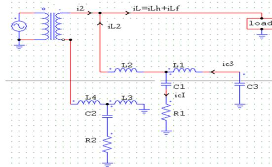
Figure(8): Equivalent circuit of the system and Fig. 6a in the case of S1, S4=on and S2, S3=off.
