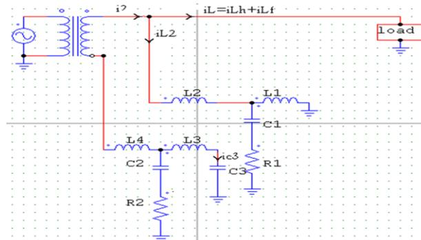
Figure(9): Equivalent circuit of the system and Fig. 6a in the case of S1, S4=off and S2, S3=on.
