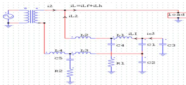
Figure(10): Equivalent circuit of the system and Fig. 6b in the case of S1=on and S2=off.
