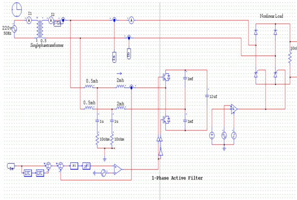
Figure(13): The block diagram of the designed system with the strategy of Fig. 6b, using the psim software.
