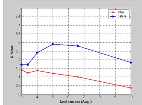
Figure(17): Variations of K factor before and after filter due to the variation of secondary currents.
