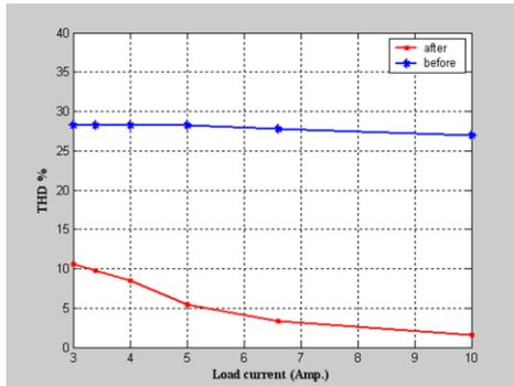
Figure(16): Variations of THDi% before and after filter due to the variation of secondary currents.
