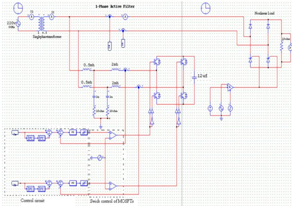
Figure (12): The block diagram of the designed system with the strategy of Fig. 6a, using the psim software.
