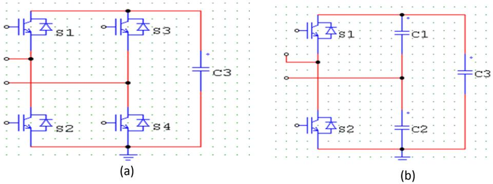
Figure(6): (a) Two branches active filter. (b) One branch active filter with two capacitors.
