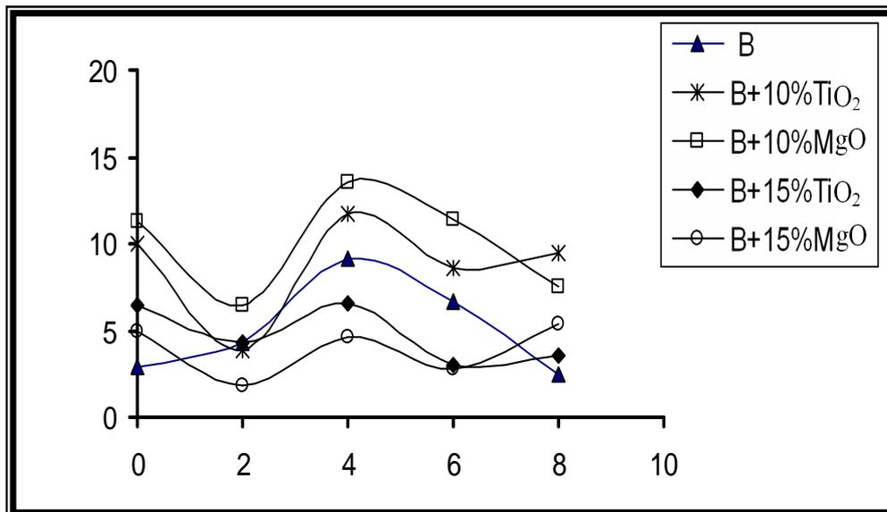
Figure (1-1): The variation in impact strength with time of immersion in water
