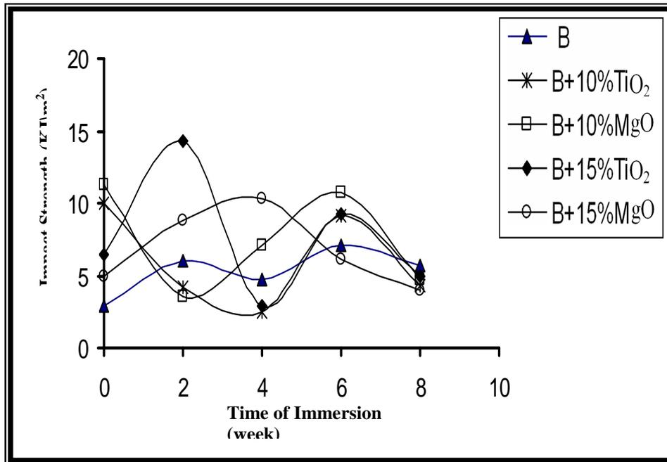
Figure (1-3): The variation in impact strength with time of immersion in HCL.
