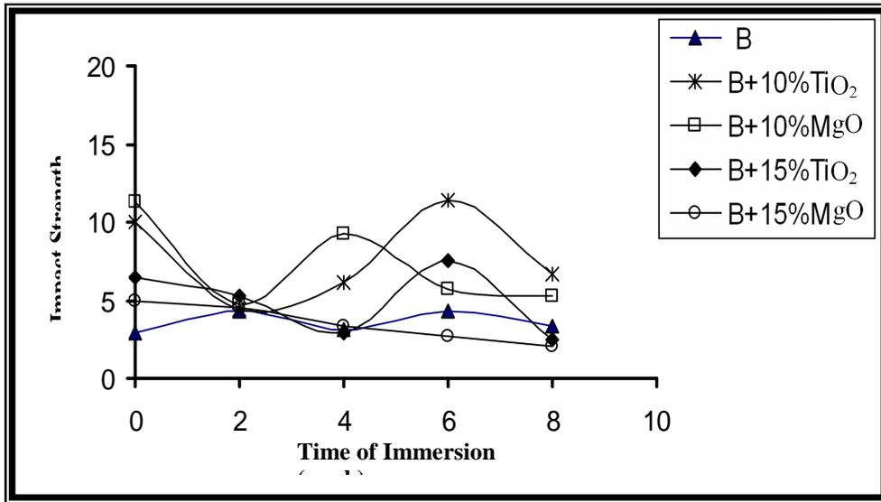
Figure (1-2): The variation in impact strength with time of immersion in KOH.
