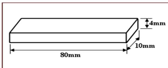
Figure 2: Standard specimens for impact test.
