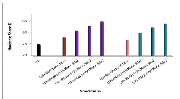
Figure 8: Hardness shore (D) for specimens composite.
