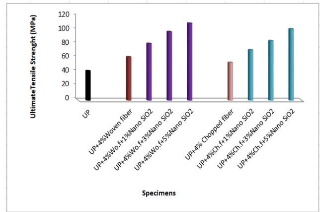
Figure 5: Ultimate tensile strength of specimens composite.
