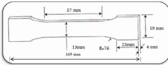
Figure 1: Standard specimens for tensile strength test
