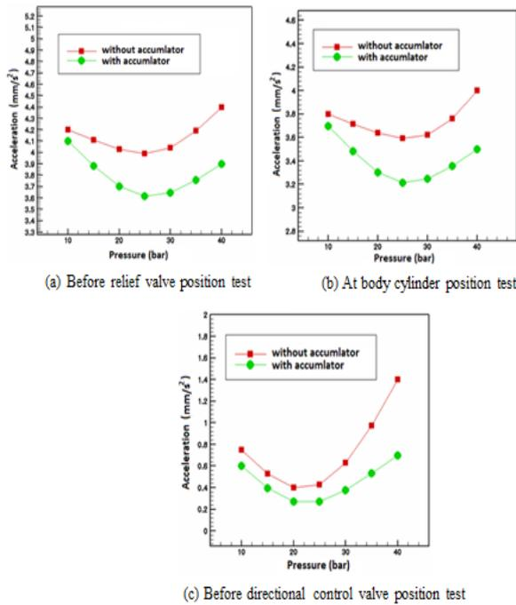
Figure 7 : Variation of Vibration Acceleration with Pressure a, b, c
