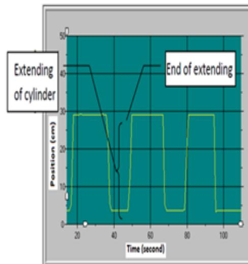
Figure 10: Extending stroke (Without accumulator)
