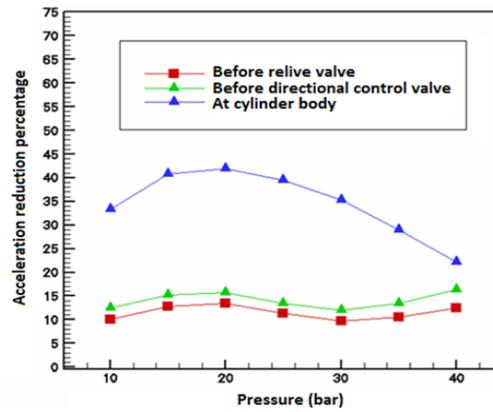
Figure 9 : Reduction percentage of acceleration with pressure
