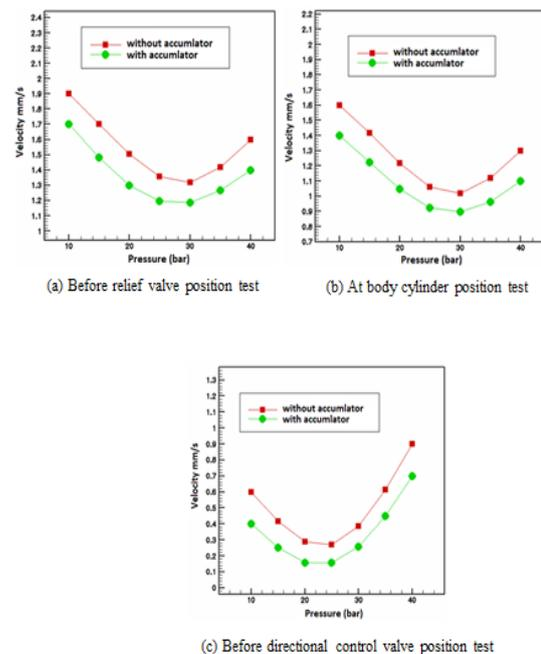
Figure 6: Variation of the Vibration Velocity with Pressure a, b, c
