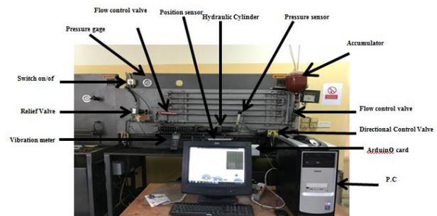
Figure 2: Experimental rig
