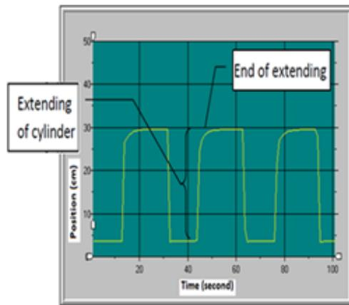
Figure 11: Extending stroke (With accumulator)
