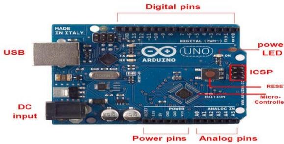
Figure 4: Arduino interface
