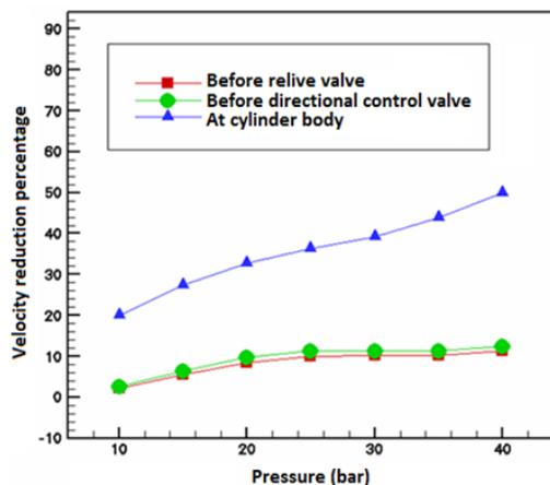
Figure 8 : Reduction Percentage of velocity with pressure
