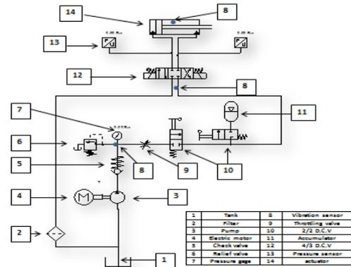
Figure 1: Apparatus schematic diagram
