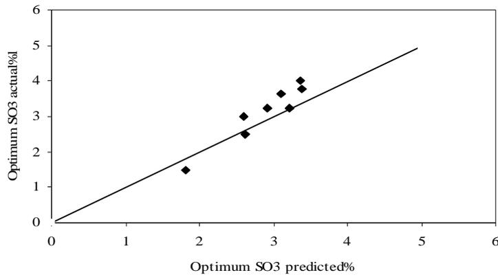
Figure (1): Relationship between optimumSO<sub>3</sub>- predicted and optimum SO<sub>3</sub>
