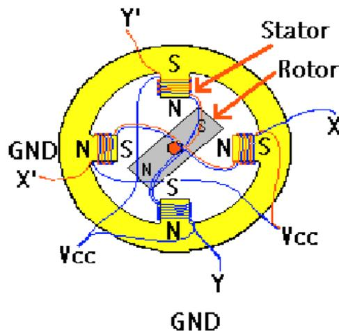
Figure (1): diagram of a stepper motor coils connection.
