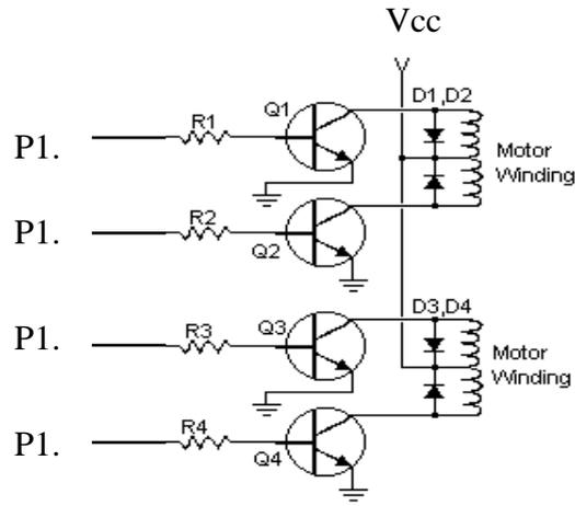
Figure (2) typical connection of transistor type stepper motor driver circuit
