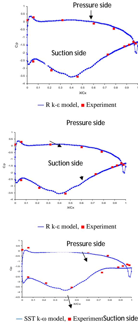
Figure (2) Comparison of  $C_p$  distributions between the experimental and CFD results
