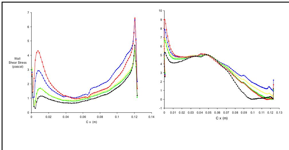
Figure (5) Wall shear stress distributions along blade pressure and suction sides
