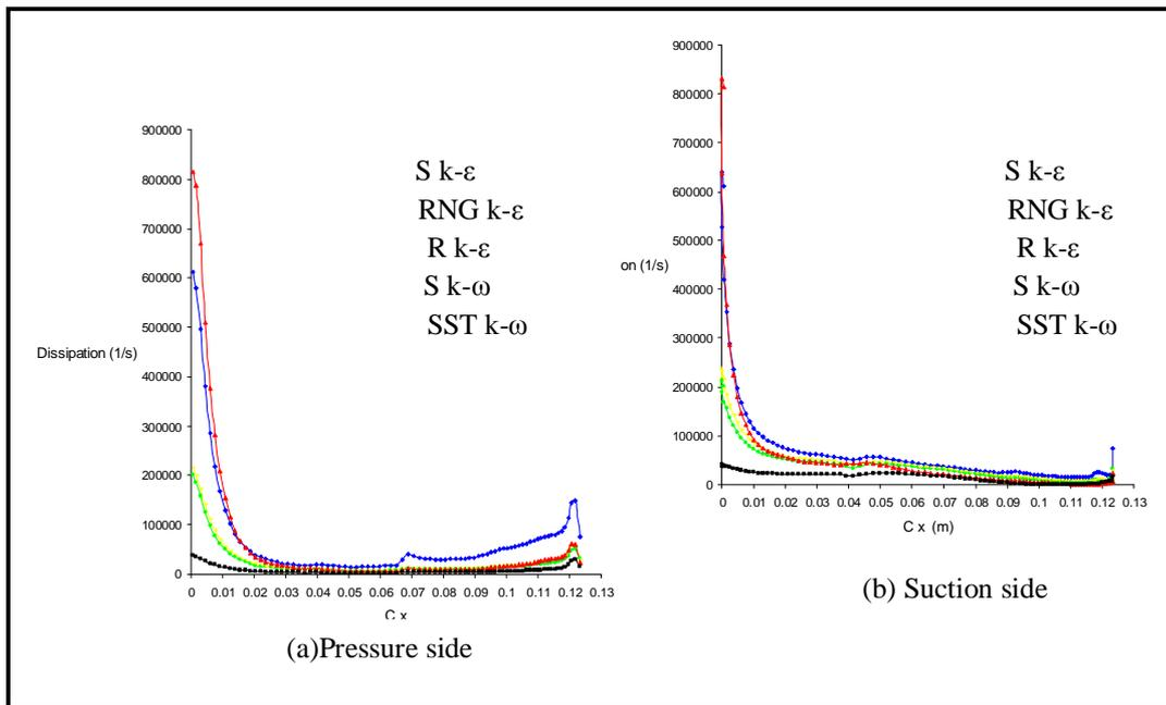
Figure (6) Dissipation rate distributions along blade pressure and suction sides suction side
