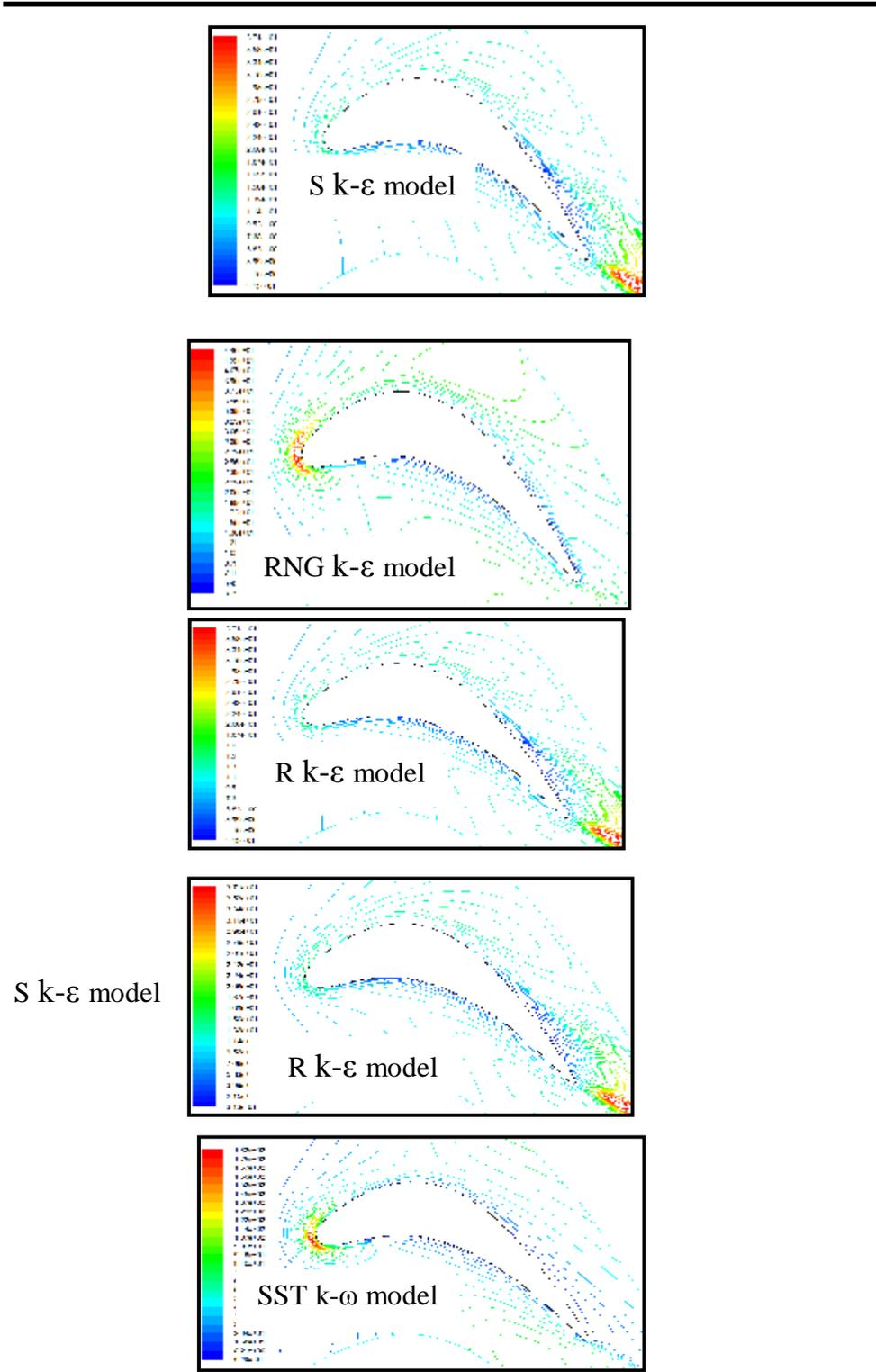
Figure (3) Distribution of turbulent kinetic energy contours around turbine blade
