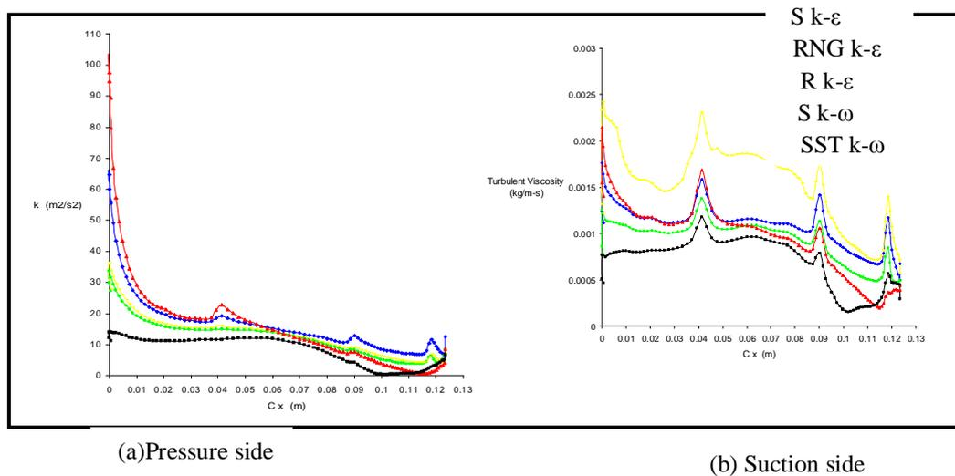
Figure (7) Turbulent viscosity distributions along blade pressure and suction sides suction side
