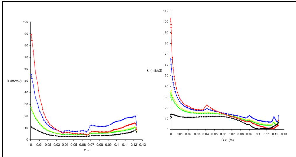
Figure (4) Turbulent kinetic energy distributions along blade pressure and suction sides
