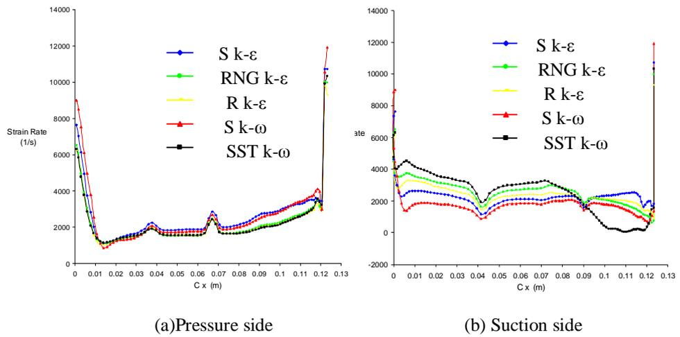
Figure (8) Strain rate distributions along blade pressure and suction sides
