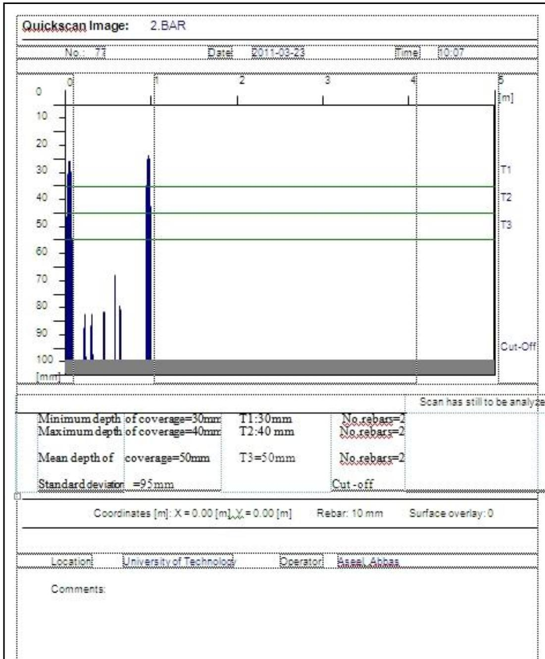
Figure (3) Details of Quick scan survey
