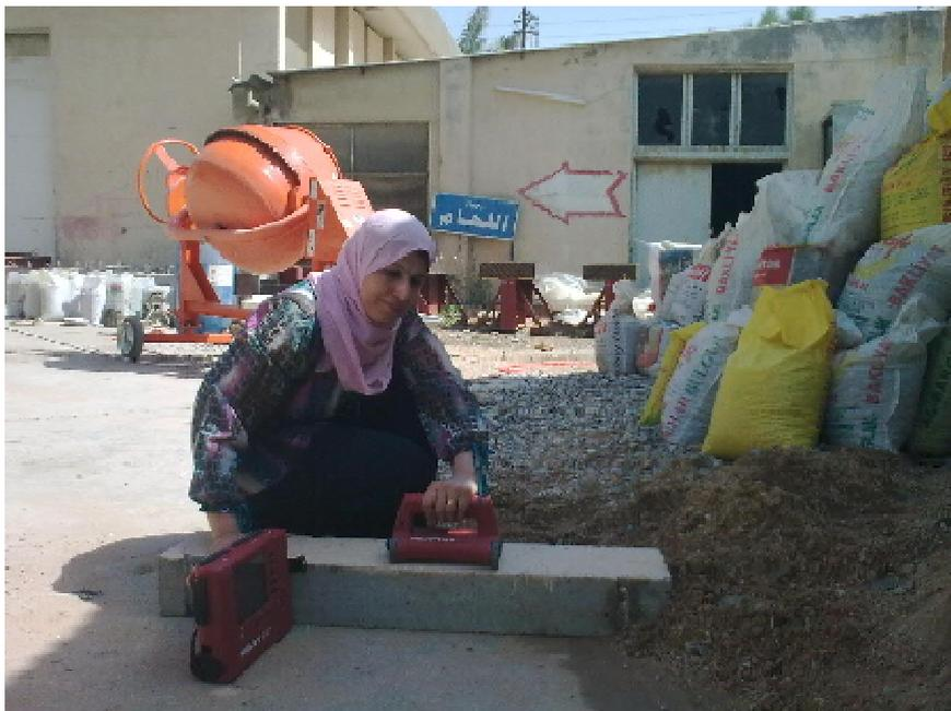
Figure (2) Testing of sample by Ferrscan
