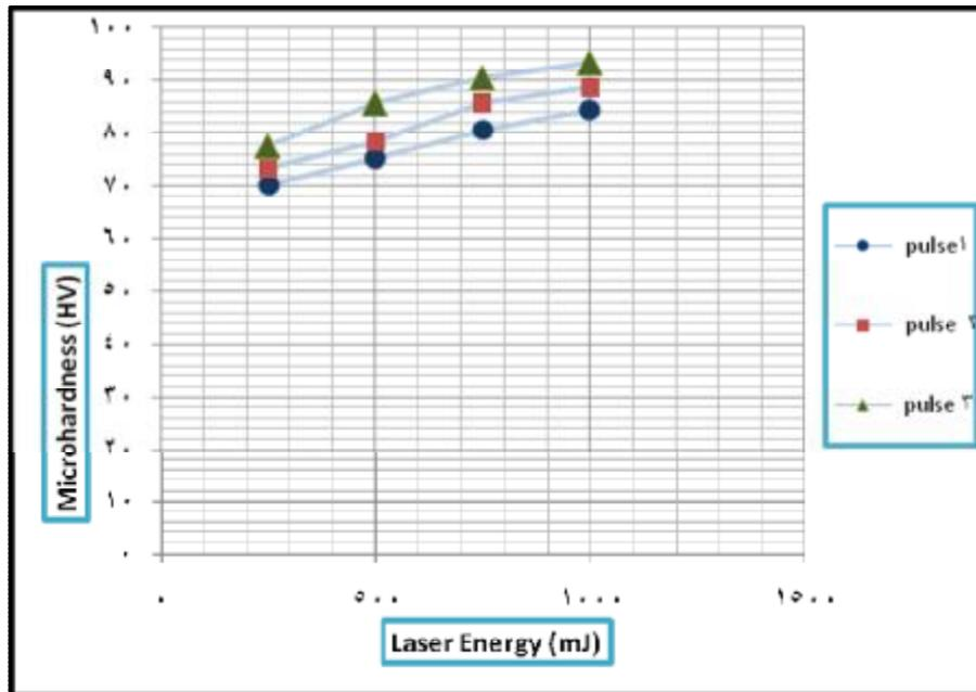
Figure( 1-9) The effect of the Laser energy and the number of shots ( pulses ) on the microhardness for samples (no.2) (Al-Si-Mg) at focal length ( $f=12$  cm ) and wavelength (1064 nm ) and spot size (1.5 mm).
