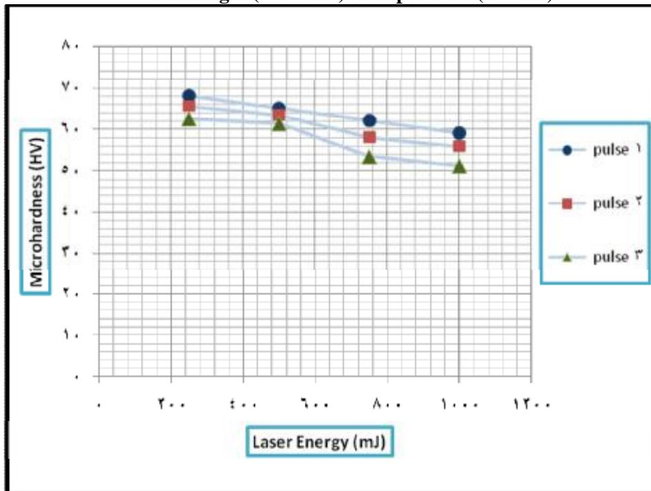
Figure(1-10) the effect of the Laser energy and the number of shots (pulses) on the microhardness for samples (no.3) (Al-Zn-Mg) at focal length ( $f=12$  cm) and wavelength (1064 nm) and spot size (1.5 mm).
