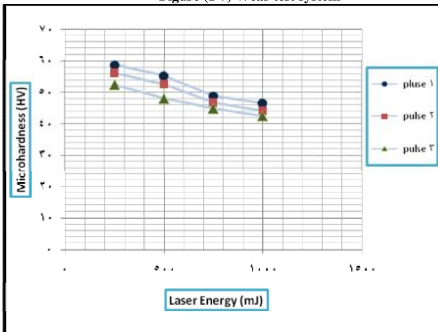
Figure (1-8) The effect of the laser energy and the number of shots(pulses) on the microhardness for samples (no.1) (Al-Cu-Si) at focal length ( $f=12\text{cm}$ ) and wavelength ( $1064\text{nm}$ ) and spot size ( $1.5\text{ mm}$ ).
