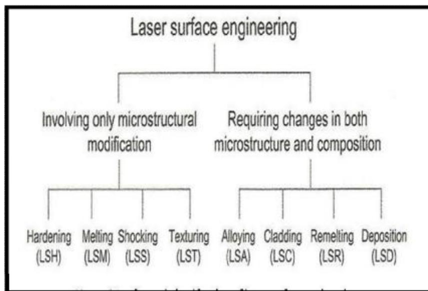
**Figure (1-1) General classification of laser surface engineering [2].**
