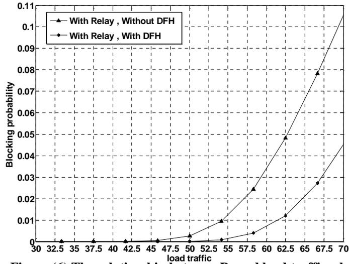
Figure (6) The relationship between  $P_B$  and load traffic when  $K = 7$ , number of calls =25 per hour, average calling time = 2 minute
