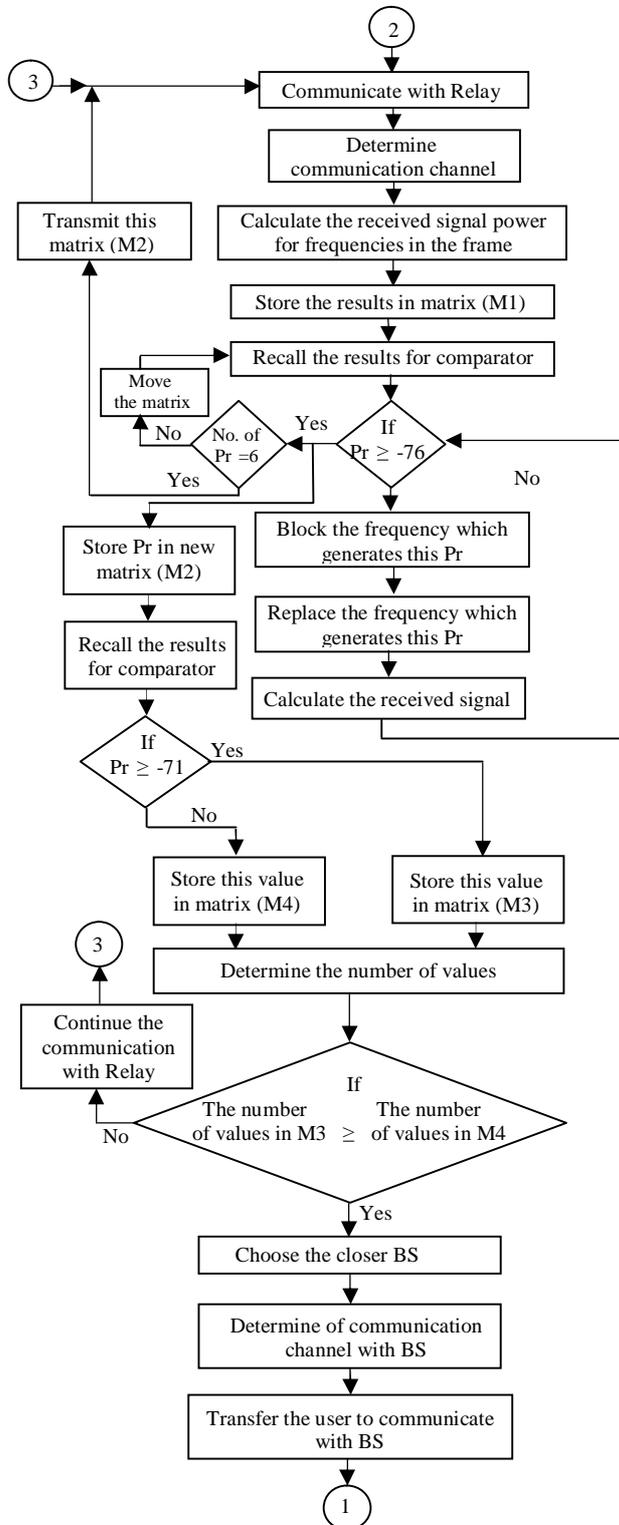
Figure (3) Simulation flowchart for operating Relay and DFH techniques in cellular system
