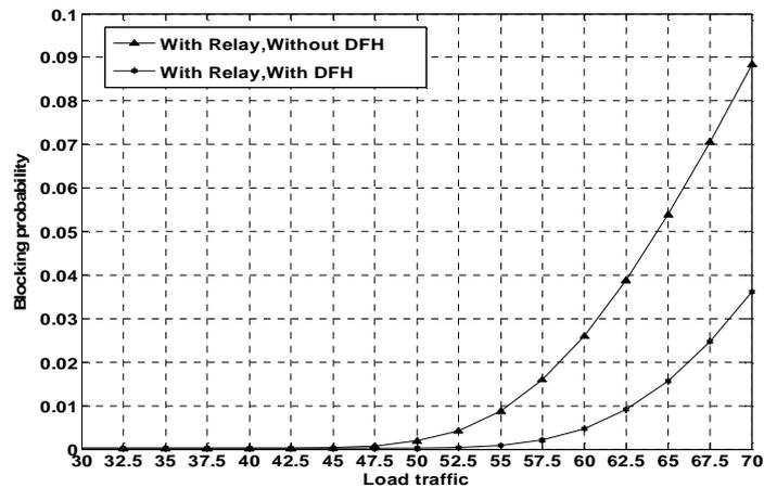
Figure (5) The relationship between  $P_B$  and load traffic when  $K = 13$ , number of calls = 15 per hour, average calling time = 2 minute
