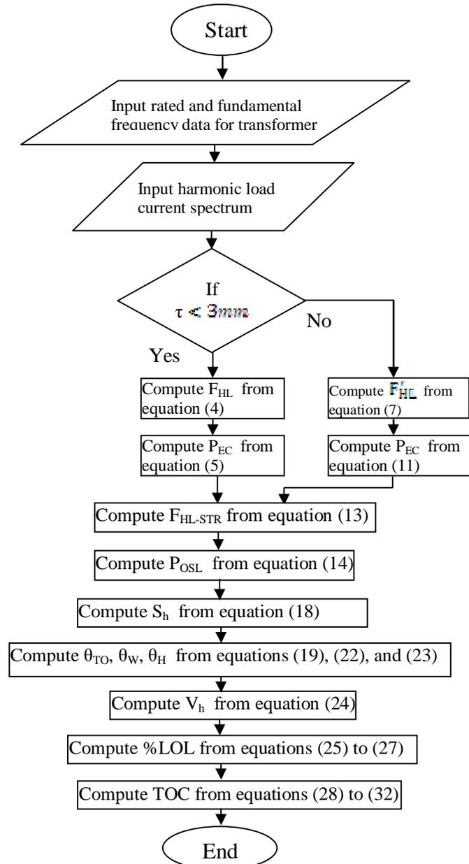
Figure (2) Flow chart of harmonic effect on power transformer algorithm
