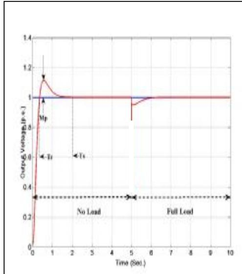
Figure (8) System Performance of GA-PID Tuning Method.
