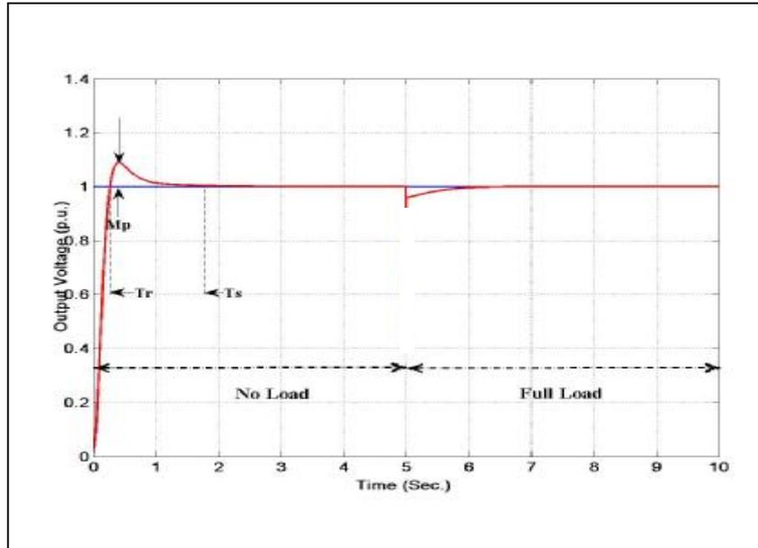
Figure (10) System Performance of PSO-PID Tuning Method.
