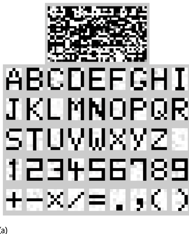
Figure (4) After training of ANN for patterns coding and compression (a) Hidden layer output (coded patterns) (b) Actual output of ANN.
