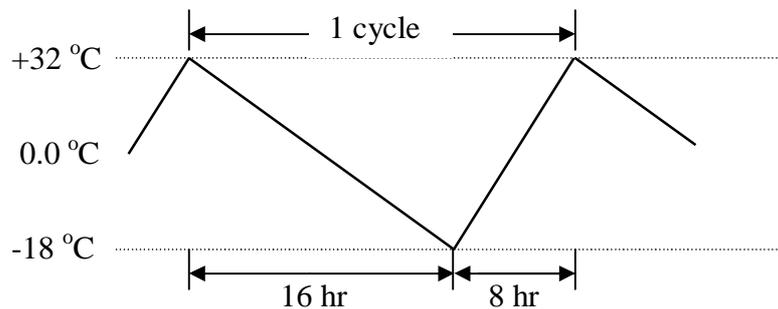
Figure (2) Schematic sketch of 1 cycle freeze-thaw test
