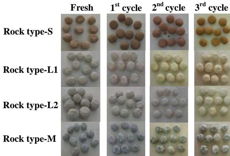
Figure (4) Changes in Shape of Specimens During Slaking Durability Test
