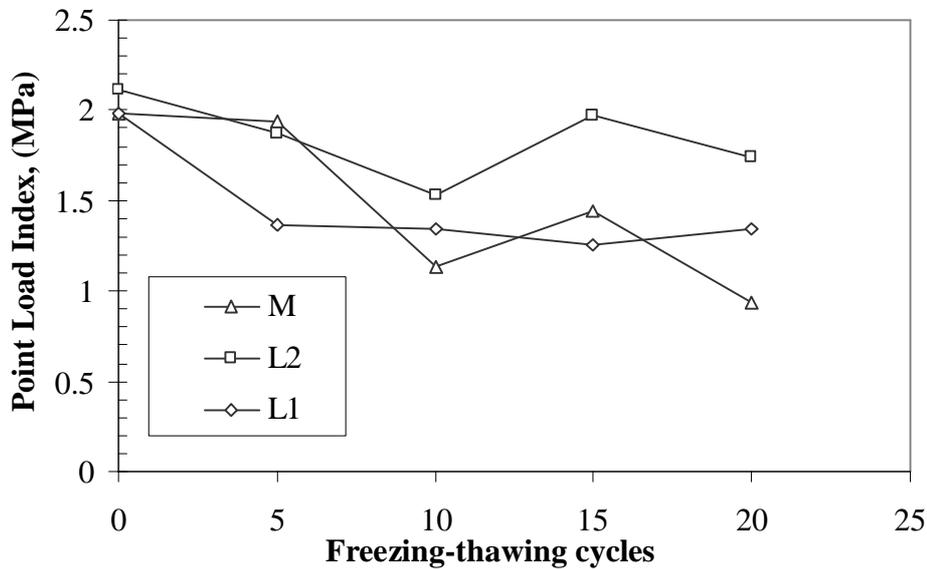
Figure (14) Effect of Freezing-Thawing Cycles on the Point Load Strength Index of the Studied Rock
