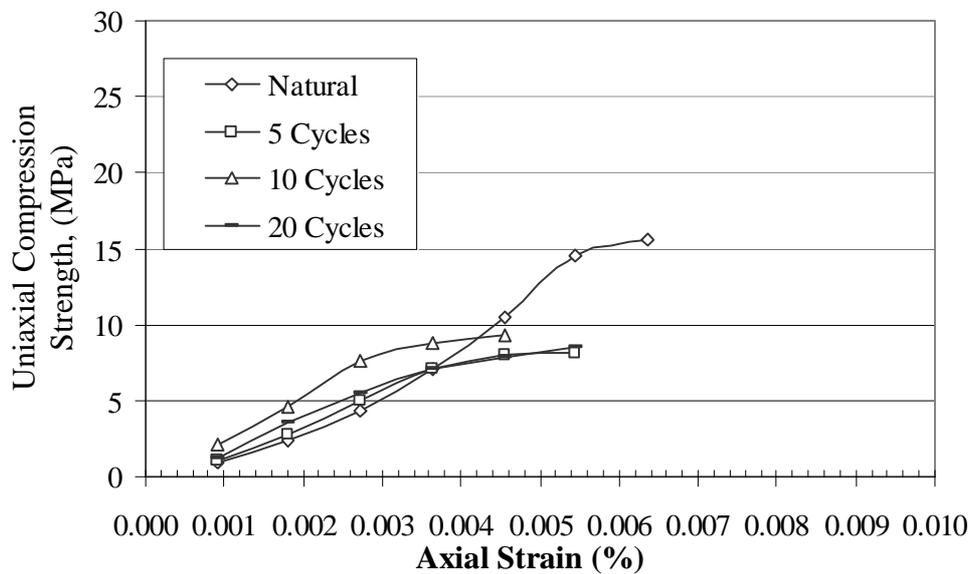
Figure (11) Effect of Freezing-Thawing Cycles on Stress-Strain Curves for Rock Type (L1)
