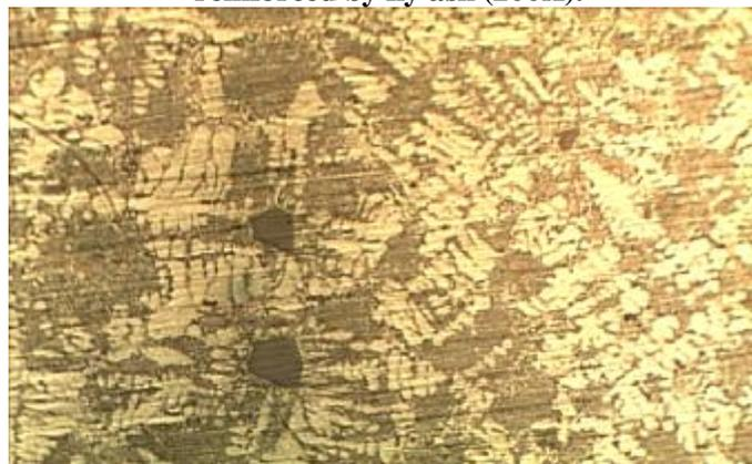
**Figure 10(b): Microstructure of metal matrix composite reinforced by dust ash (200X).**
