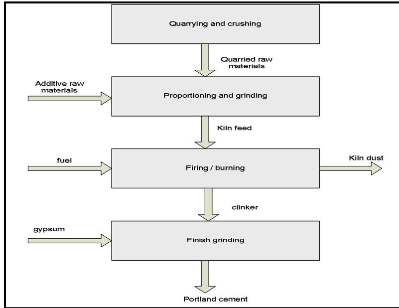
Figure (1) Basic flow diagram of the Portland cement manufacturing process (USEPA, 1993) [3].
