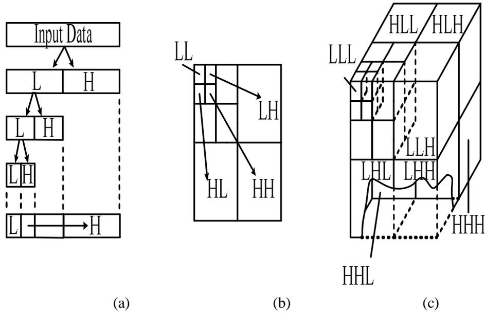
**Figure (4) Hierarchical structure of the wavelet coefficients:**
