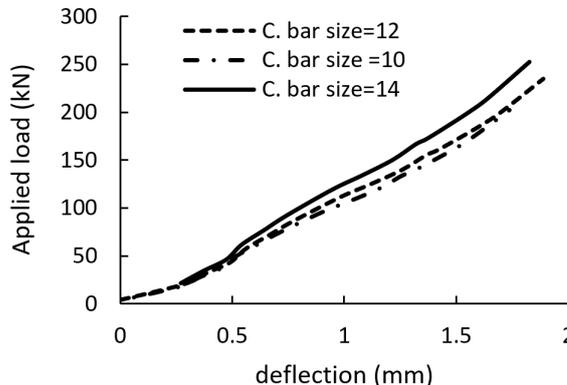
Figure 9. Conventional cyclically loaded beam with different steel reinforcement sizes.
