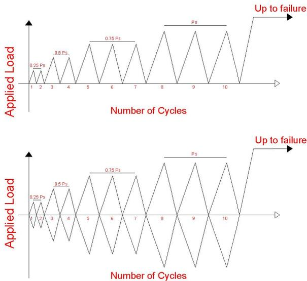
Figure 3. Simulated reverse cyclic load using ANSYS APDL.
