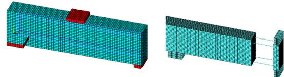
Figure 5. The Concrete, Supports and bearing plate meshing and Steel rebars.
