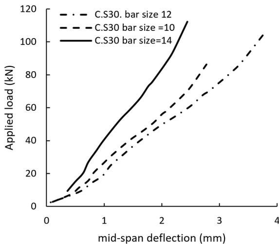
Figure 10. Fine aggregates rubberized concrete beams under cyclic load for different reinforcement amounts.
