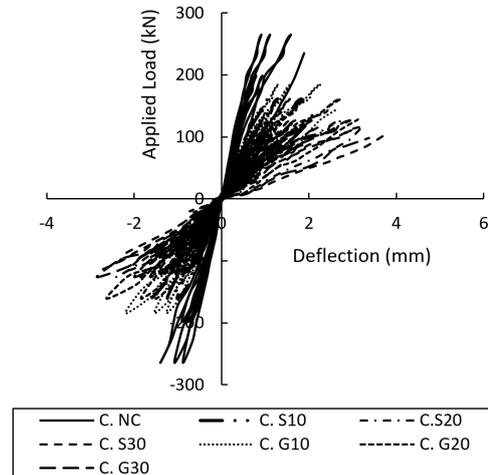
Figure 6. Load versus deflection curves for all specimens under cyclic loadings.
