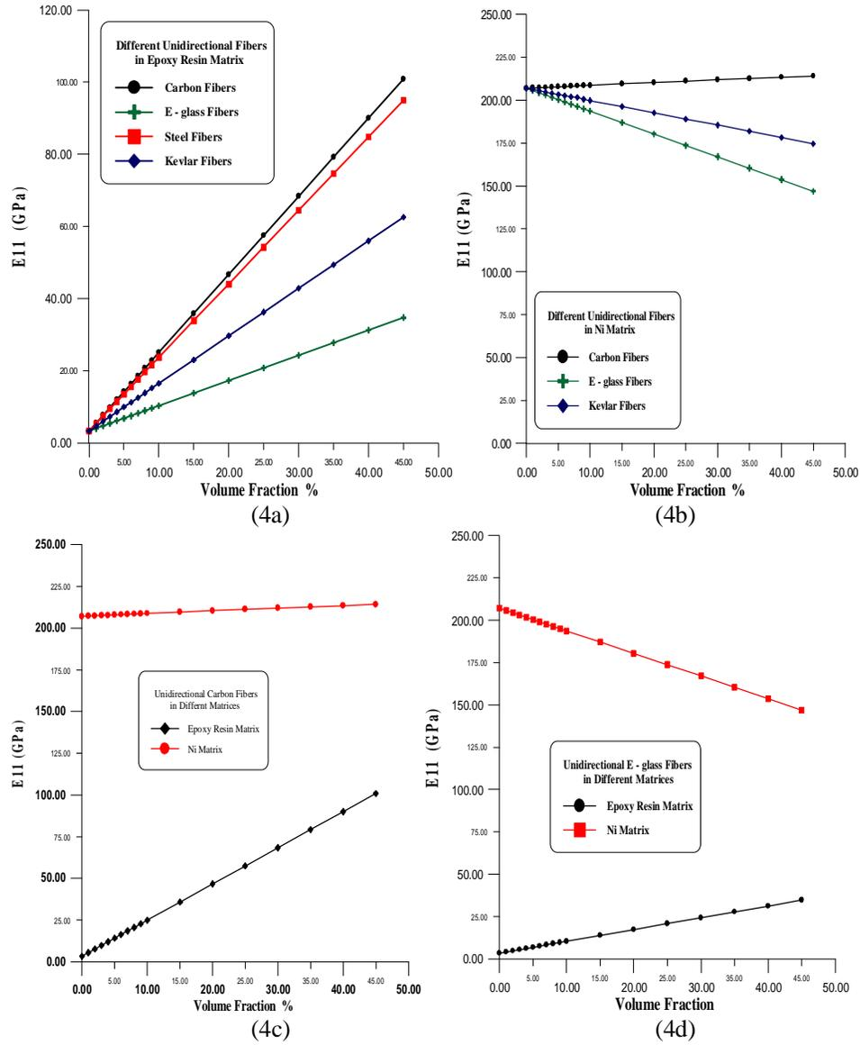
Figure (4)  $E_{11}$  comparison of different unidirectional fibers embedded in different matrices
