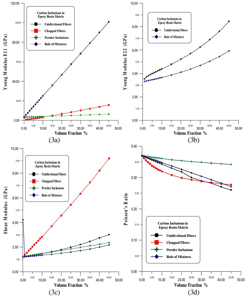
Figure (3) Mechanical properties comparison for Carbon Inclusions in Epoxy Resin Matrix
