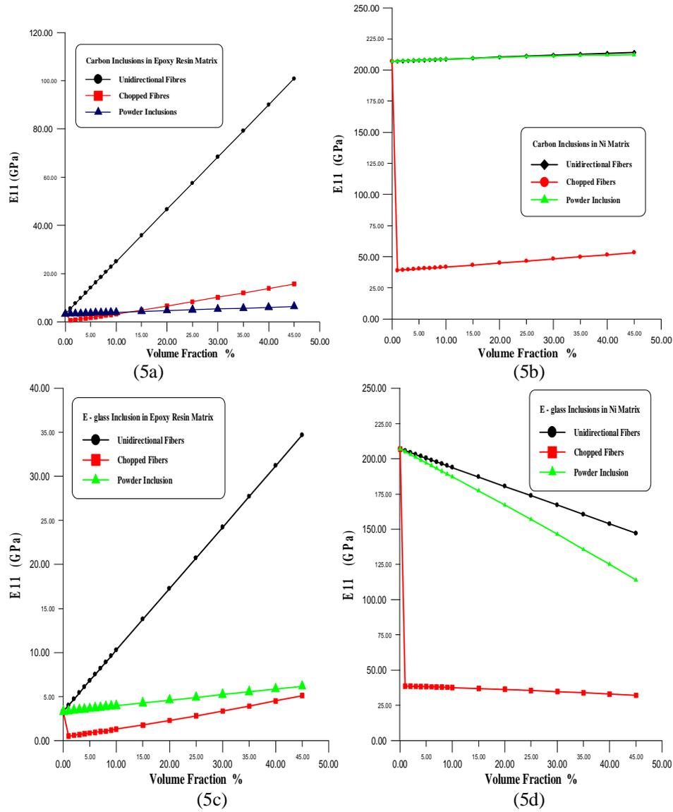
Figure (5)  $E_{11}$  comparison of different inclusions embedded in different matrices
