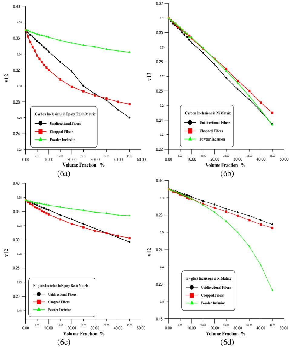
Figure (6) Poisson's Ratio comparison of different inclusions embedded in different matrices
