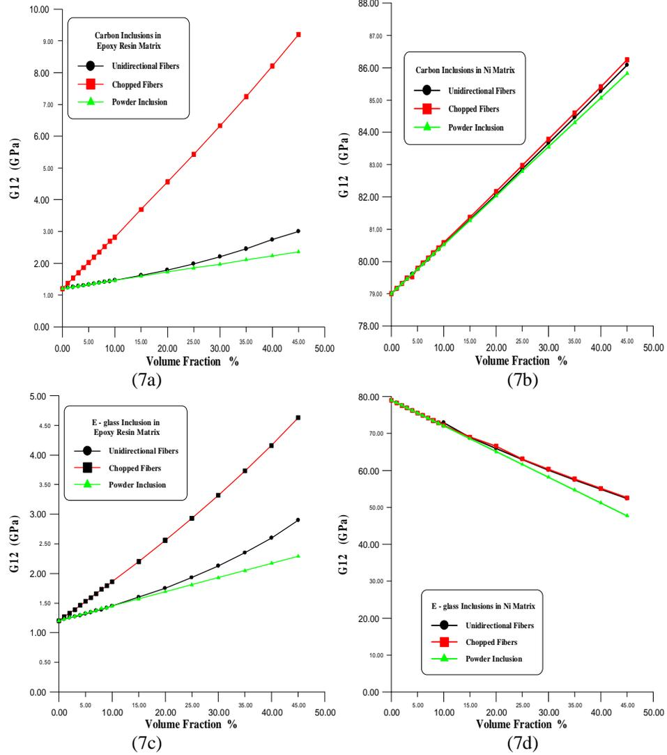
Figure (7) Shear Modulus comparison of different inclusions embedded in different matrices
