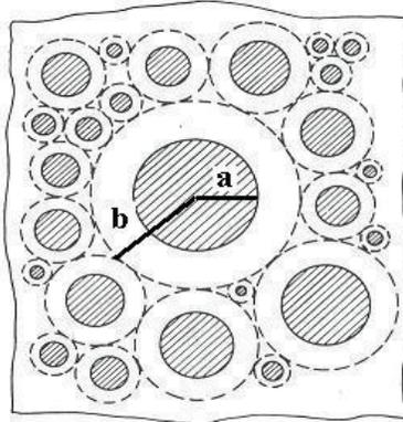
Figure (1) Composite sphere assemblage
