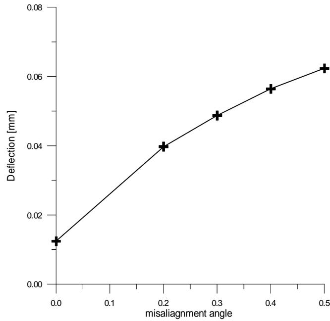
Figure (17) The relationship between the misalignment angle and the deflection on spur gear
