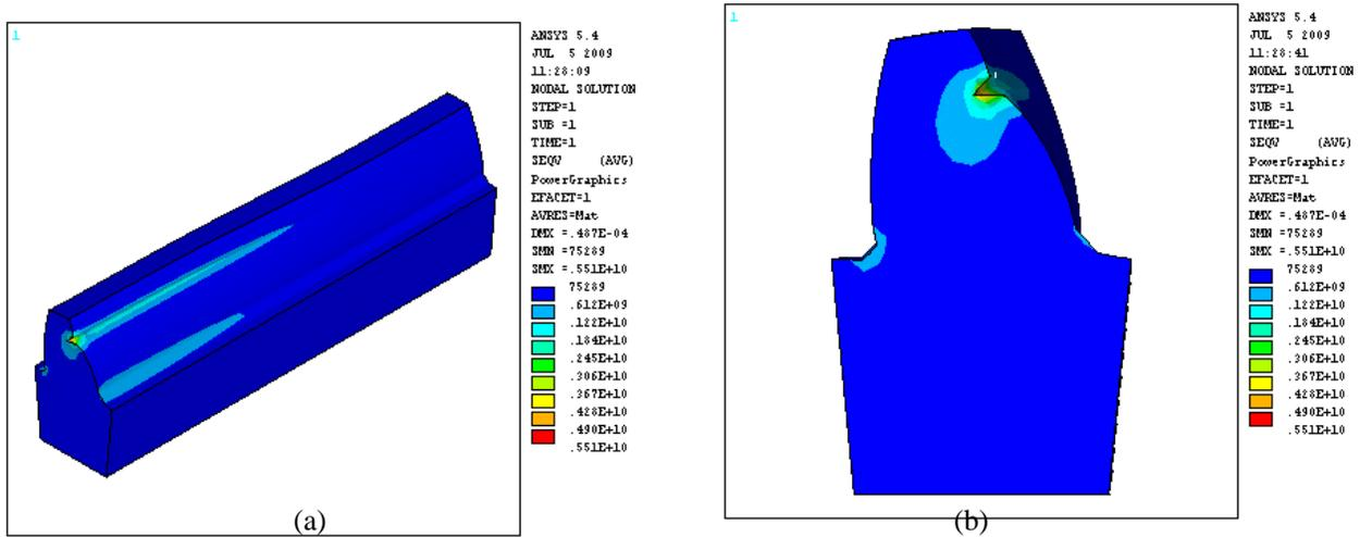
Figure (13) Explain the stress distribution on the gear width when  $\alpha = 0.3^\circ$
