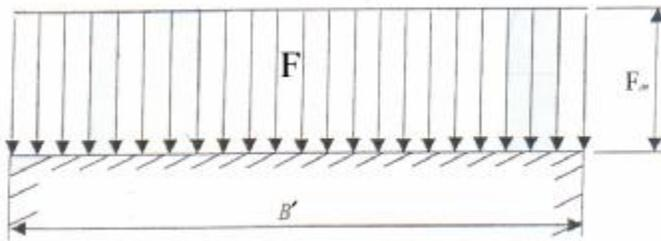
Figure (2) Uniform distributed of load in along the gear width
