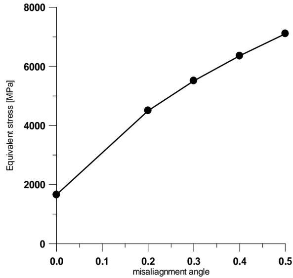
Figure (16) The relationship between the misalignment angle and the equivalent stress on spur gear
