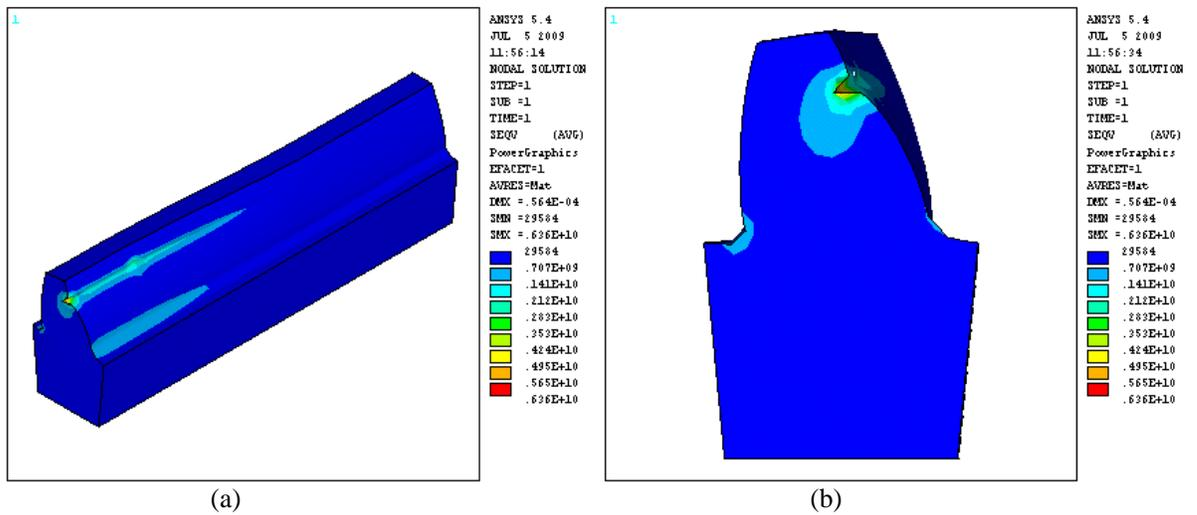
Figure (14) Explain the stress distribution on the gear width when  $\alpha = 0.4^\circ$
