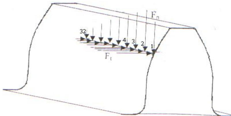
Figure (7) The components of equivalent forces for misalignment gear
