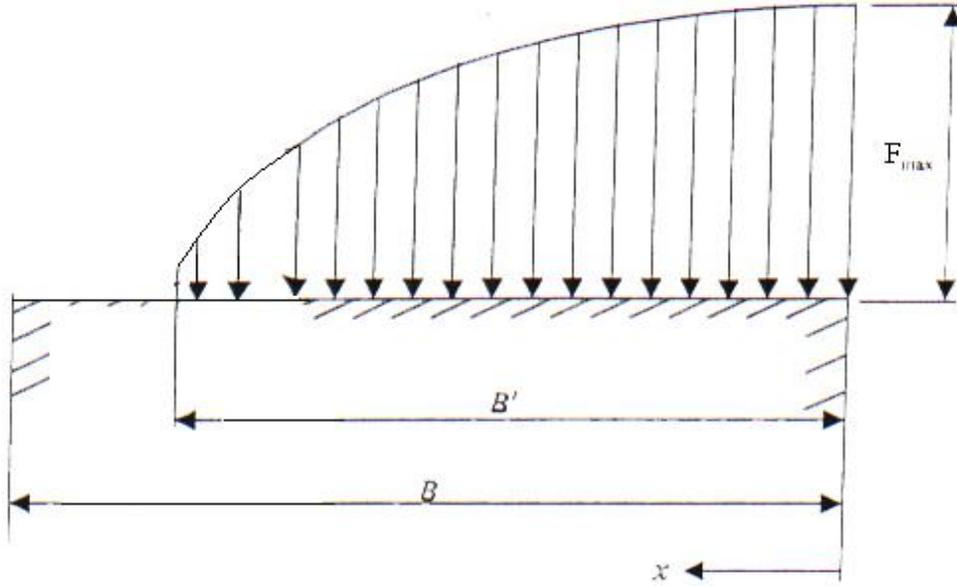
Figure (4) Load distribution along the active gear width in contact when misalignment is occur
