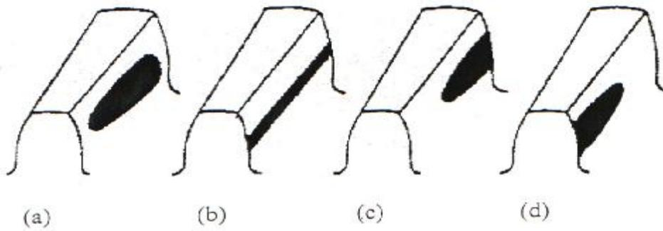
Figure (5) Configurations of load the regions on the tooth face during misalignment
