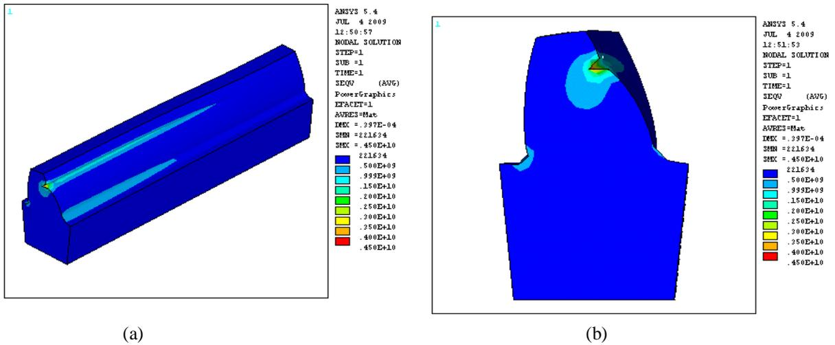
Figure (12) Explain the stress distribution on the gear width when  $\alpha = 0.2^\circ$
