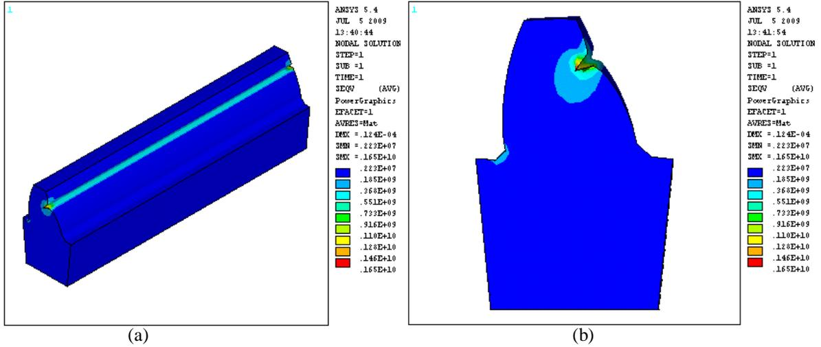
Figure (11) Explain the stress distribution on the gear width when  $\alpha = 0^\circ$
