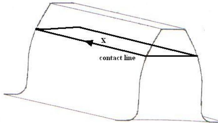
Figure (6) Configurations of the contact line between the gearing tooth
