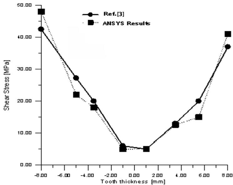
Figure (18) The relationship between the tooth thickness and shear stress when misalignment angle = 0
