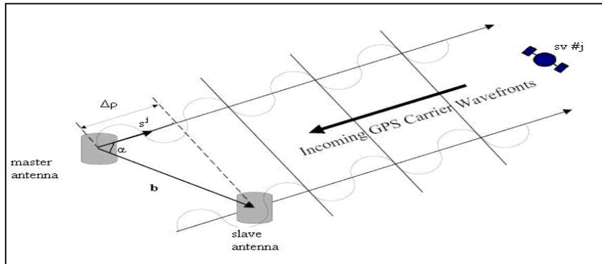
Figure (1) Interferometric Model.
