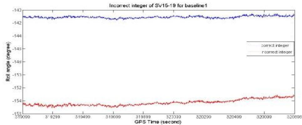
Figure (8c) Roll Estimation Using Incorrect Integer.
