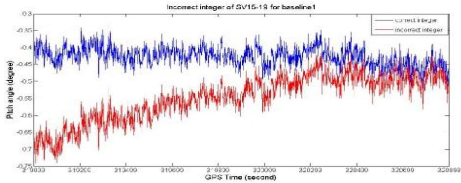
Figure (8b) Pitch Estimation Using Incorrect Integer.
