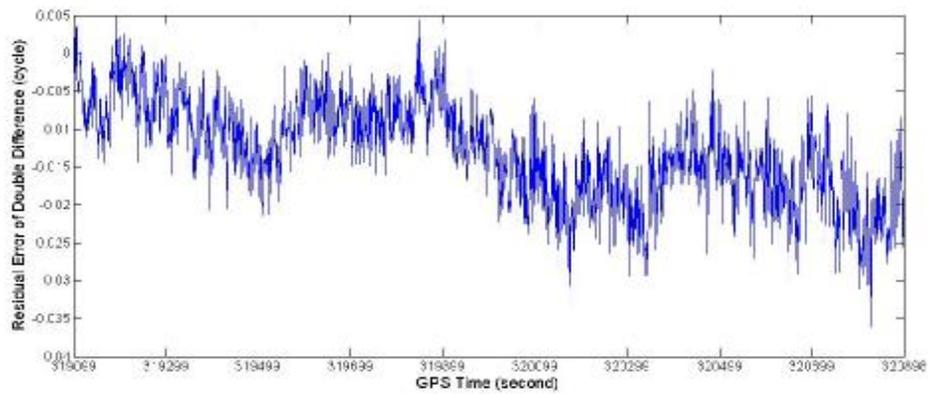
Figure (7e): The Residual Error of  $\Delta\nabla\tilde{\Phi}_2^{15-21}$
