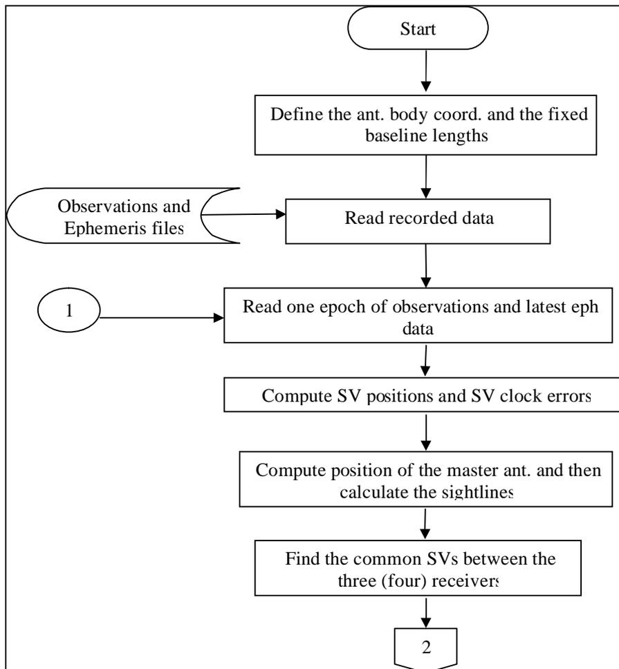
Figure (2) The Flowchart of the Attitude Determination system
