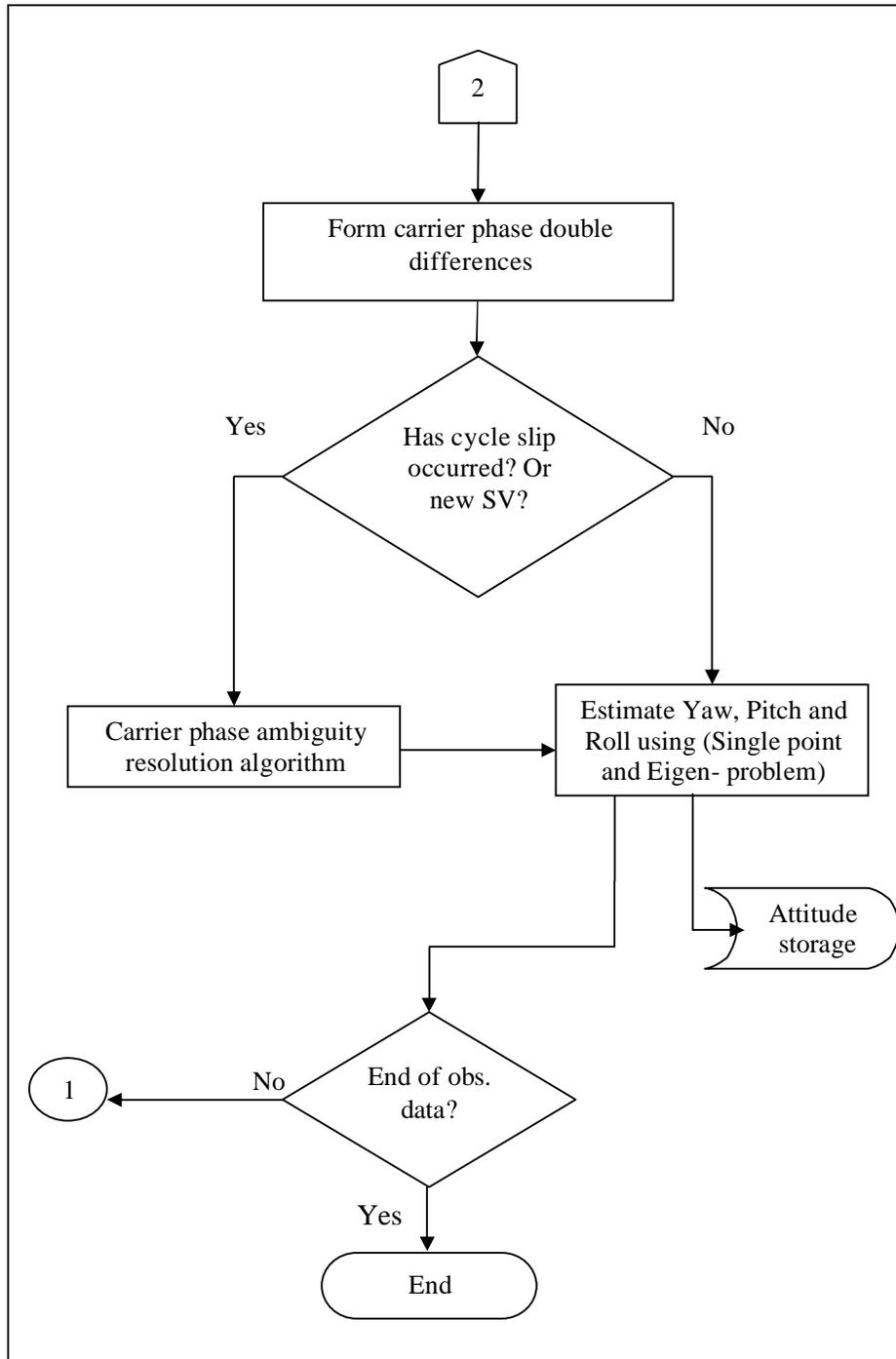
Figure (2) The Flowchart of the Attitude Determination system (continued).
