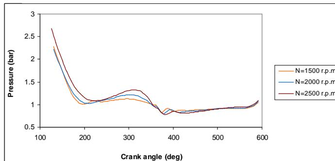
Figure ( 9 ) Pressure variations inside the cylinder during gas exchange period at different speeds with CR =9.
