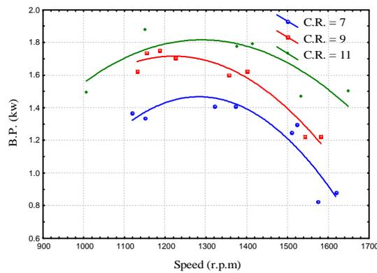
Figure (3) Effect Variable Compression ratio
