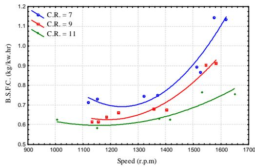
Figure ( 4) Effect Variable Compression ratio on Brake Specific Fuel Consumption as a Function of Engine
