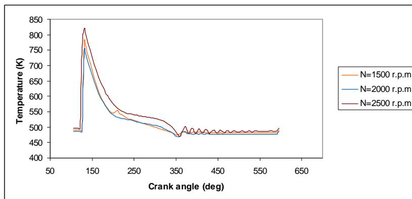
Figure (14) Temperature variations in the exhaust pipe during gas exchange period at pipe end no.1.
