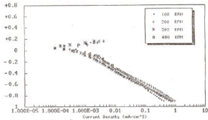
Figure (5) Potentiostatic Polar. Curve of Inhibited Oxygenated Sol., Temp.298K
