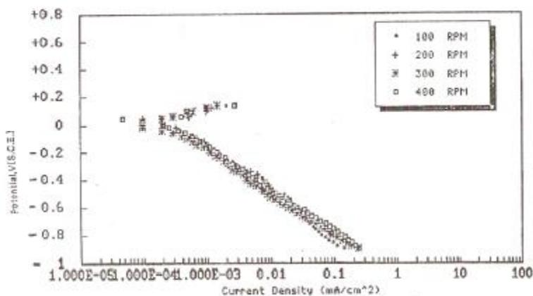
Figure (2) Potentiostatic Polar. Curve of Inhibited Oxygenated Sol., Temp.283K
