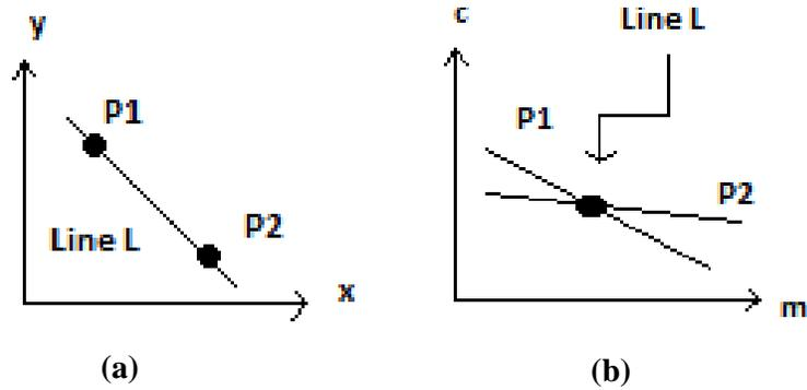
Figure (3) (a) Points on the same line, and (b) The mapping of P1 and P2 from Cartesian space to the (m,c) space.
